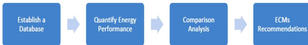
*Figure 2-1: Building Energy Benchmarking Process*
