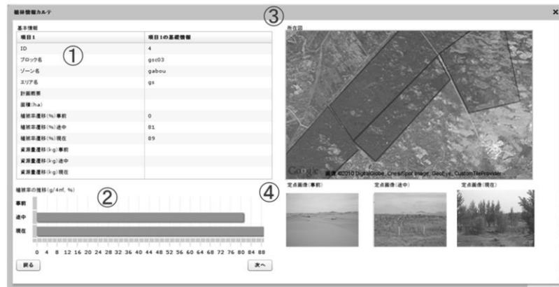
Fig.6-5 WebGIS based interface for data visualizing. ① Basic information, ② Vegetation coverage graph, ③ Target location image, ④ Fixed point image. Each detail was shown above.
