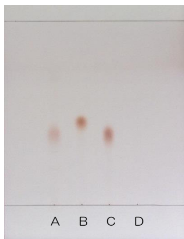
Fig. 3-5 TLC comparison of glucose, galactose, sorbitol and hydrolysate of 11a . solvent system; 2-propanol/methanol/water (6:2:1), detection; spraying thymol-sulfuric acid-methanol TS for spraying then heating at 105°C for 5 minutes. A: hydrolysate of 11a ; B: glucose; C: galactose, D: sorbitol
