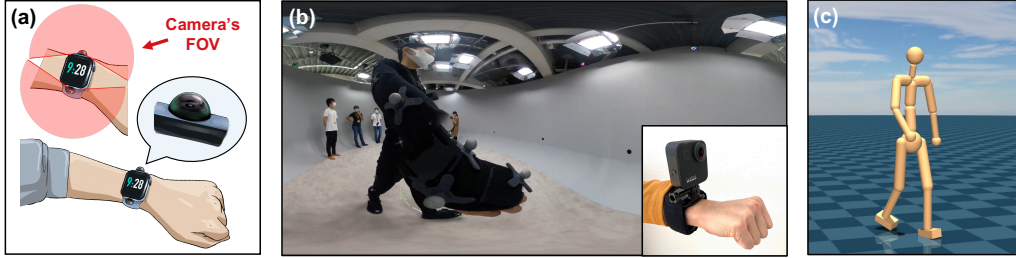
Figure 3.1: Concept of our 3D human pose estimation method using a wrist-mounted 360° camera. (a) Future vision depicting a smartwatch with a 360° camera. The area shown in red represents the camera's field of view; (b) Camera view with a 360° camera (GoPro MAX) mounted on the wrist, which is the camera configuration of our method; (c) 3D pose of the user estimated from (b) image by our 3D human pose estimation framework.
