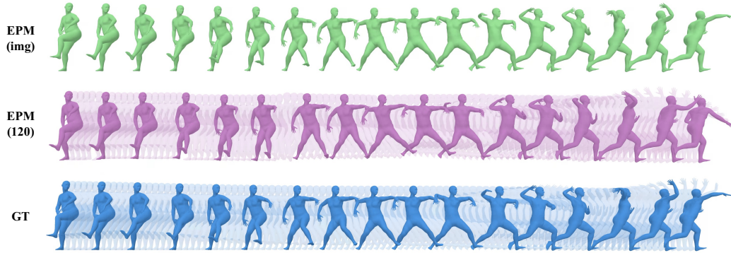
Figure 4.9: Qualitative results of the Task2 described in Sec. 4.3.5. The topmost “EPM(img)” represents our method’s results when segmenting events according to the intensity image frame rate, which varies with the lighting conditions. The middle “EPM(120)” shows the outcomes when segmenting events and estimating the meshes at the same 120fps. The bottom “GT” shows the ground truth meshes with a frame rate of 120fps. Note that the transparent meshes in the bottom two rows are only for visual clarity; there is no difference from the opaque meshes.
