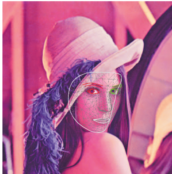
Figure 4.10. An example of face mesh extracted from the image that contains a face using Media Pipe.
