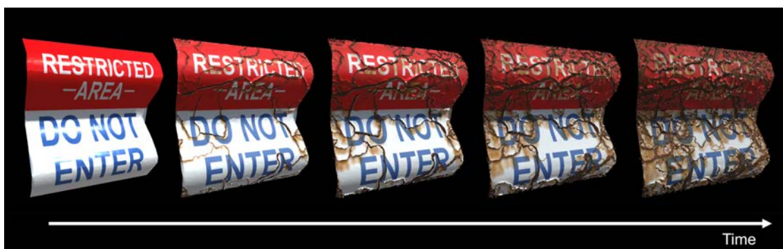
Fig. 9.1 A result of weathering a coated curved plate. As time progresses, cracks and bends are generated
