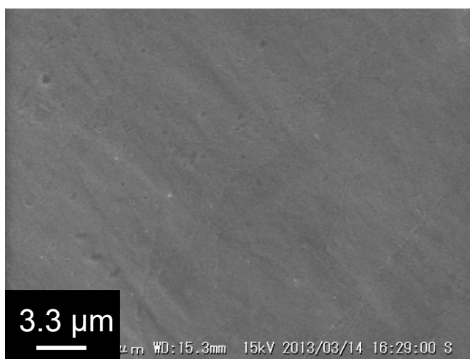
Fig. 2-28 SEM image of the Ni electrode with LiPON thin film after Li deposition and dissolution in 1 M LiTFSA/BMPTFSA. Surface was washed with DME and exposed in air.
