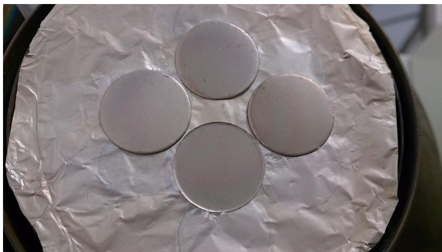
Fig. 2-12 Image of surface of the Ni substrate after Ar gas sputtering.
