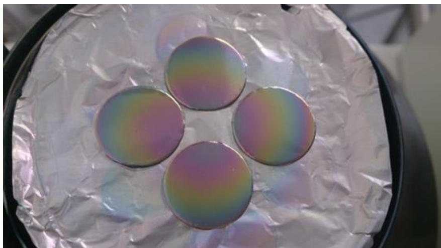
Fig. 2-13 Image of surface of the Ni substrate after N 2 gas sputtering.
