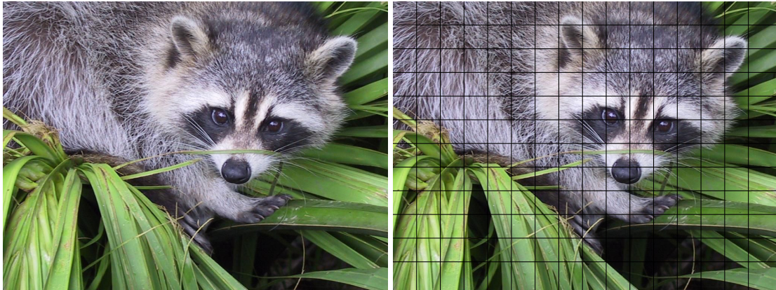
Figure 2.5: Illustration of centroid initialization in SLIC when the number of initial superpixels is 192. The left image denotes an input image, and the right image denotes the boundary of initial superpixels. The centroid has the mean position and color of the pixels contained in each grid.
