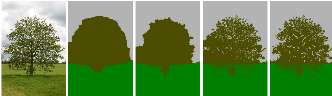
Figure 2.1: Example results of various CRF-based semantic segmentation methods. From left to right, an input image, grid CRFs [Shotton et al., 2009a], robust P^n CRFs [Kohli et al., 2009], fully connected CRFs [Krähenbühl and Koltun, 2011], and ground truth. The results are taken from [Krähenbühl and Koltun, 2011].
