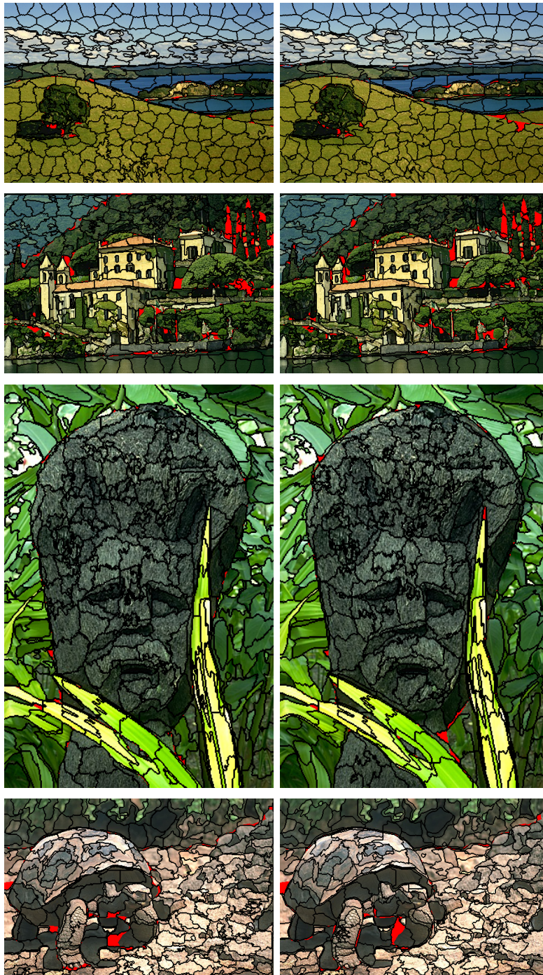
Figure 5.12: Example results of the HCSSN (left) and the SSN (right). Red regions denote the undersegmentation error [Stutz et al., 2018] that measures the “leakage” of superpixels with respect to ground truth labels. Thus, the images with fewer red areas are better.
