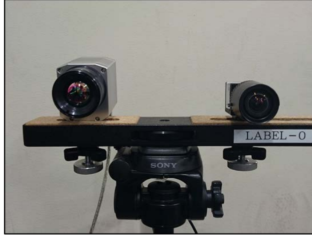
Figure 3.11: Camera rig. Left: thermal-infrared camera. Right: RGB camera.
