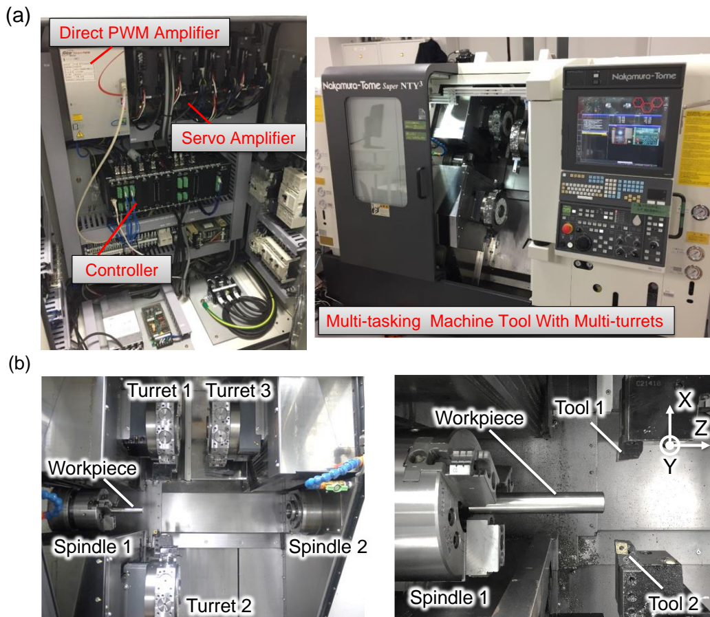
Fig. 5-8 Prototype multi-tasking machine tool: (a) external appearance (b) workspace view
