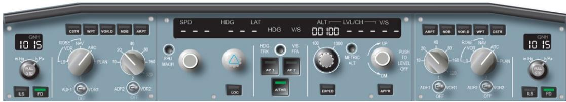
**Figure 2.4** Glareshield panel of the Airbus A320 showing the FCU in the center <sup>(38)</sup>
