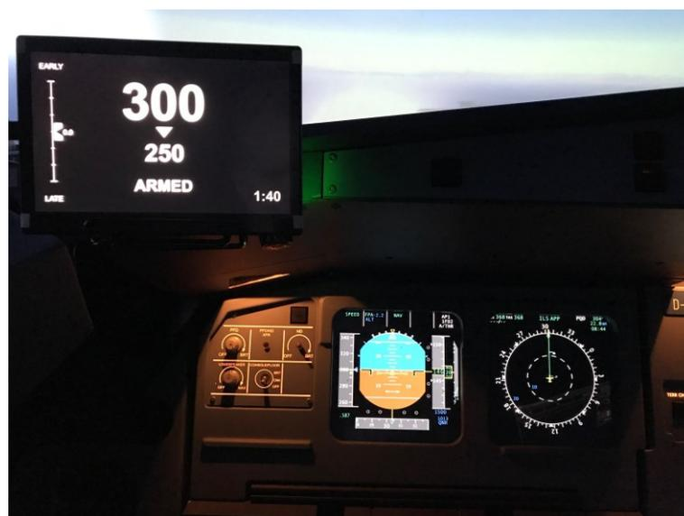
**Figure 6.2** Position of the CGD on the Captain's side <sup>(59)</sup>
