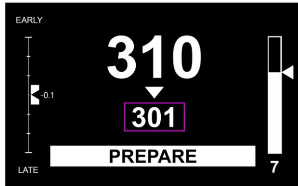
**Figure 6.8** GUI B indicating a speed plan change that requires immediate crew reaction
