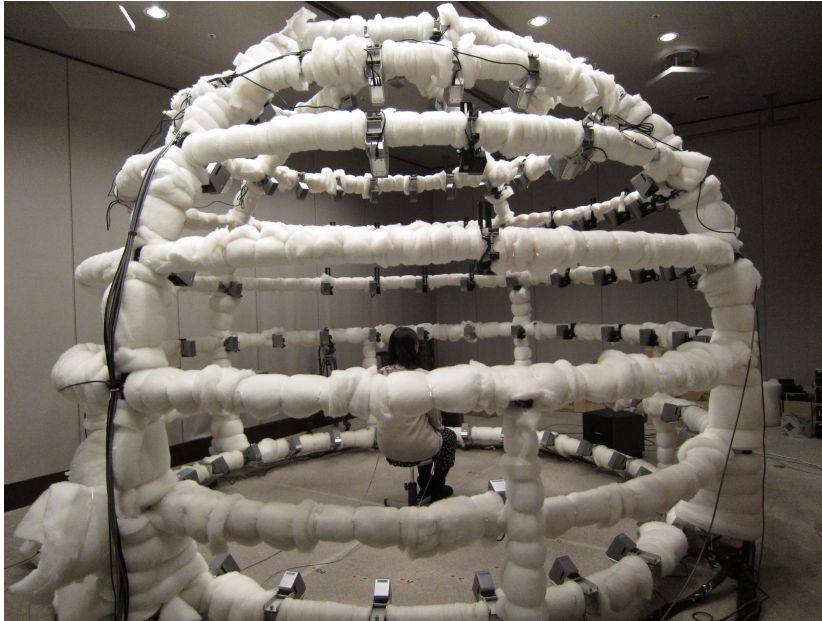
Fig. 3.3: Measurement of impulse responses for simultaneous estimation in a sound proof room of the NHK Science and Technology Research Laboratories
