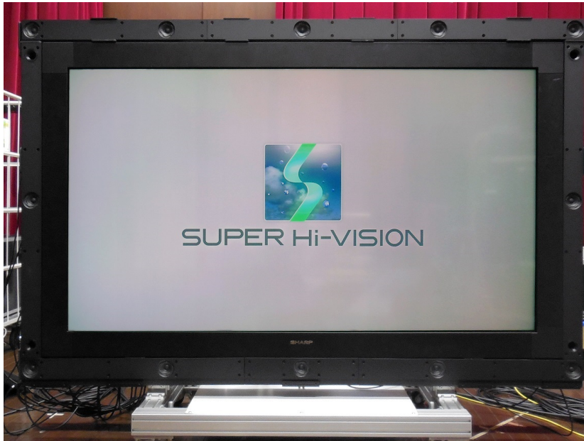
Fig. 5.5: 12-loudspeaker frame integrated into an 85-inch LCD jointly developed by NHK and Foster Electric Company, Ltd.
