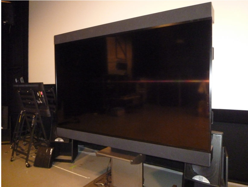
Fig. 5.8: Digital line array loudspeaker jointly developed by NHK and Sharp Corp.
