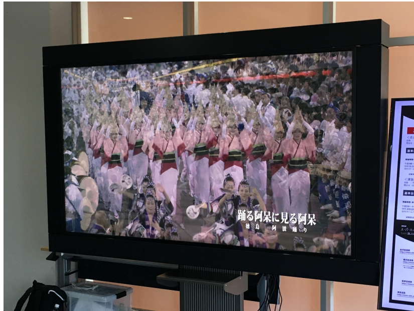
Fig. 5.7: Digital loudspeaker frame jointly developed by NHK and Sharp Corp.
