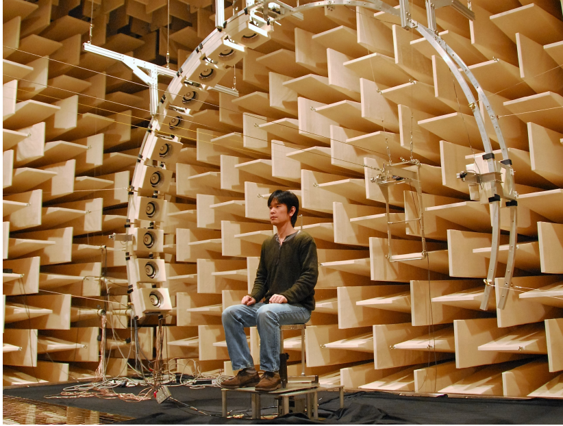
Fig. 2.5: Measurement of impulse responses in an acoustic anechoic chamber of the NHK Science and Technology Research Laboratories
