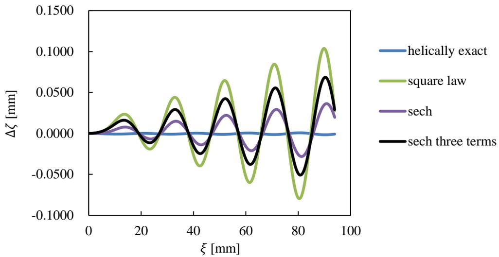
**Figure 7-10** The difference of  $\zeta$  between the calculation of exact ray path and algorithm B with different refractive index distribution with  $\zeta_i = 0.2$  mm,  $\eta_i = 0.0$  mm. Used refractive index profiles were helically exact distribution, square low profile, meridionally exact or secant hyperbolic distribution, and secant profile approximated as three terms.
