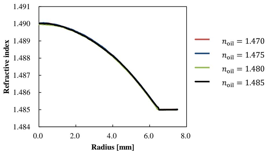
**Figure 5-19 Numerical refractive index profile of convex GI waveguide.**
