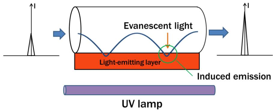
Figure 2-6 Model of optical amplifier with N-GI-POF.
