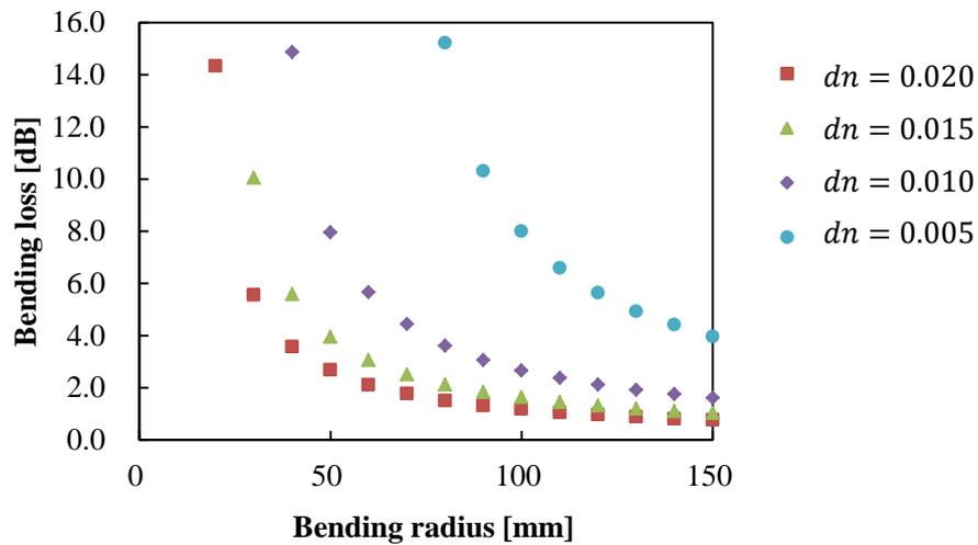
Figure 4-14 Numerical bending loss of in each curvatures about several refractive index difference ( $dn = 0.020, 0.015, 0.010, 0.005$ ).
