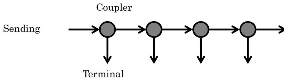
Figure 2-5 Schematic representation of bus in network.
