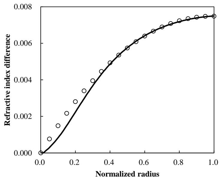
Figure 6-11 Refractive index profile of the preform rod fabricated using UV laser. Plot indicates approximated profile ( $g = 2.0$ ).
