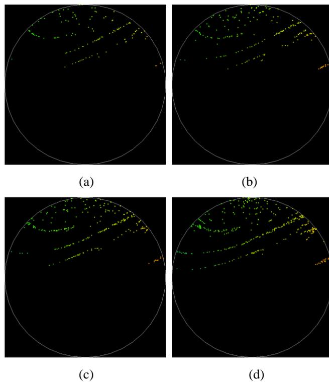
**Figure 7-34** The position of input rays that transferred fiber (N-GI waveguide, (a)  $d = 0.01$  mm, (b)  $d = 0.02$  mm, (c)  $d = 0.03$  mm, (d)  $d = 0.05$  mm).
