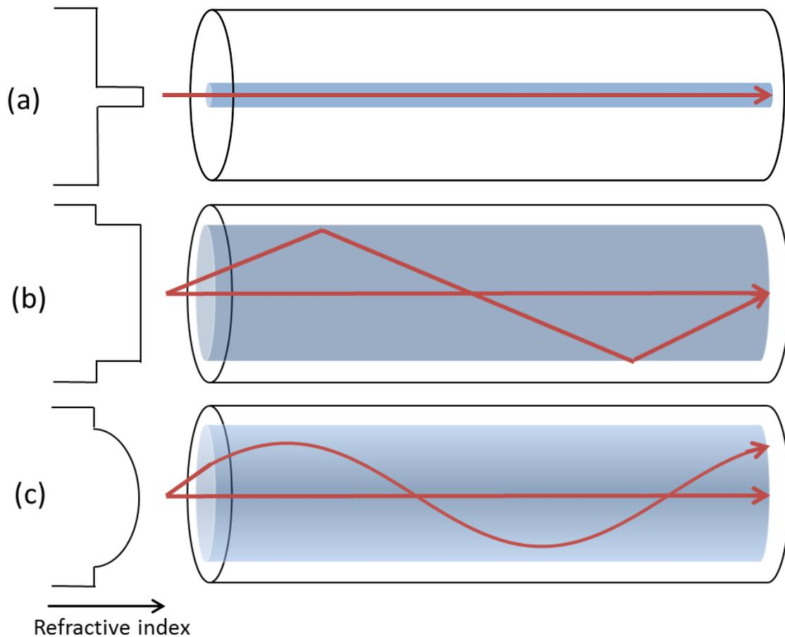
**Figure 2-1 Refractive index profile and trajectory of ray of several types of optical fiber. (a)SM fiber, (b) SI fiber (c) GI fiber.**
