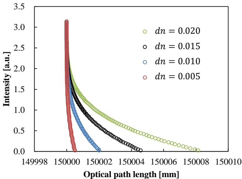
Figure 3-16 The dependence on  $dn$  of optical path length and intensity of light in two-terms refractive index distribution.
