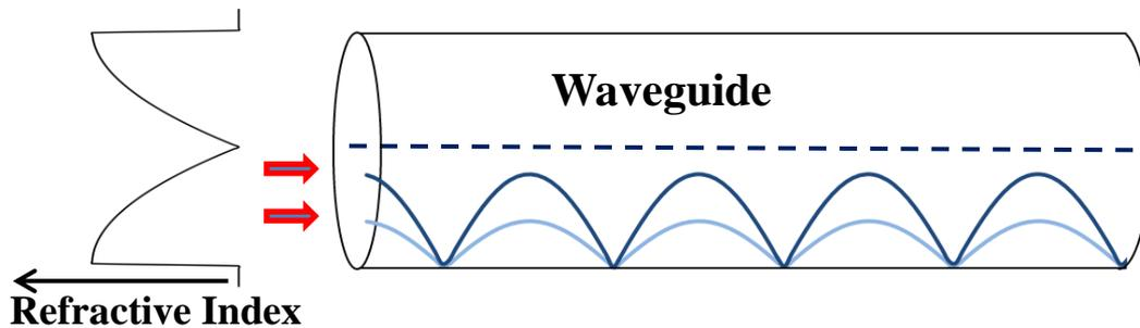
**Figure 2-3 Schematic representation of the shape of refractive index distribution and trajectory of ray in negative type GI waveguide.**
