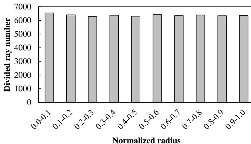
Figure 4-5 Divided ray number and distance from center of waveguide to starting ray position.
