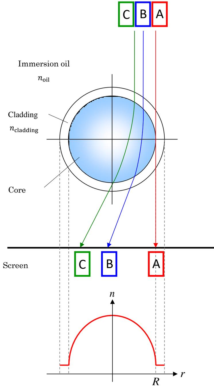
Figure 5-1 Ray trajectory inside GI-POF.
