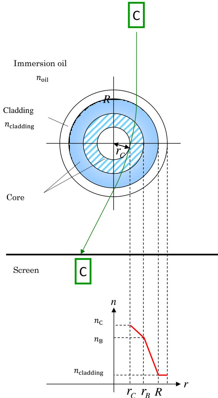
Figure 5-3 Determination of the refractive index profile by ray C.
