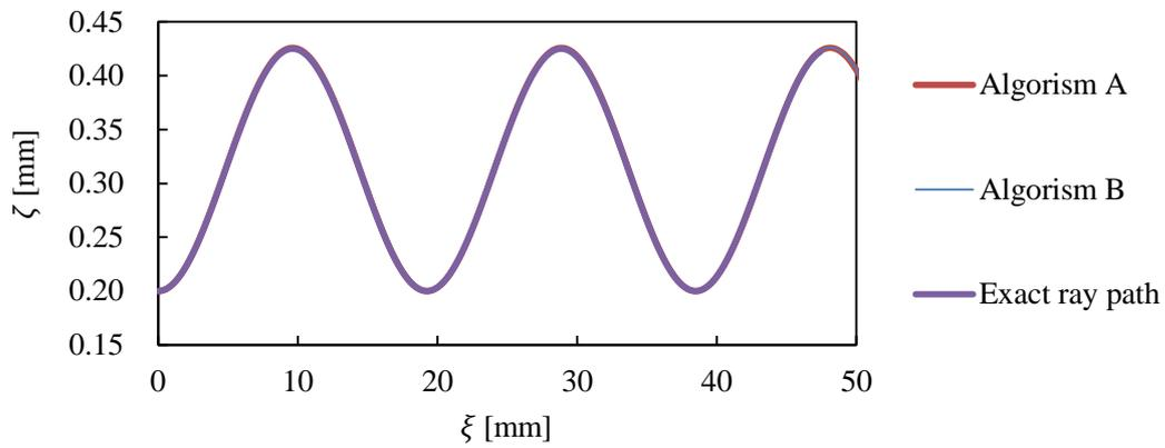
**Figure 7-9 Ray position of  $\zeta$  along  $\xi$  gave by calculation of exact ray path, algorithm A, and algorithm B with  $\zeta_i = 0.2 \text{ mm}$ ,  $\eta_i = 0.0 \text{ mm}$ .**
