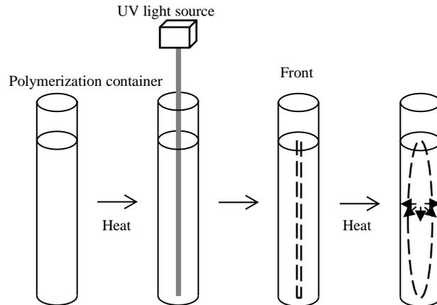
Figure 6-1 Schematic representation of UV-assisted frontal polymerization technique.
