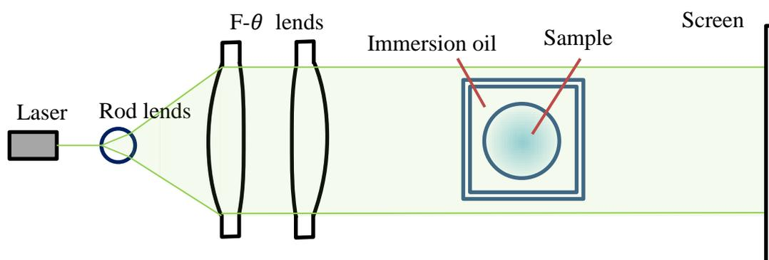
Figure 5-4 Experimental configuration of the system to determine the refractive index profile.
