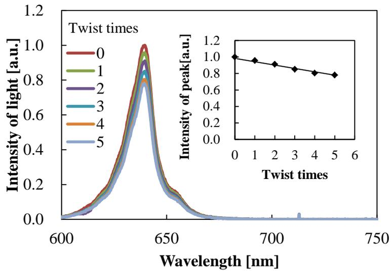
Figure 6-15 Output light spectra of original fiber with twist times. Inset indicates the transition of intensity peaks.
