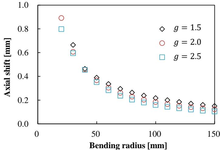
Figure 4-18 Axial shift of passed region in different  $g$  ( $g = 1.5, 2.0, 2.5$ ).
