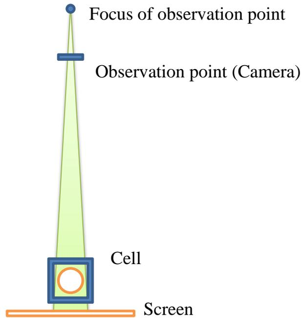
Figure 5-8 Schematic representation configuration of novel system to determine the refractive index profile.
