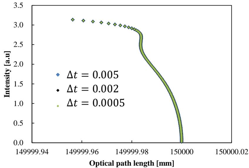
Figure 3-6 Optical path length and intensity with different  $\Delta t$  in convex GI waveguide.
