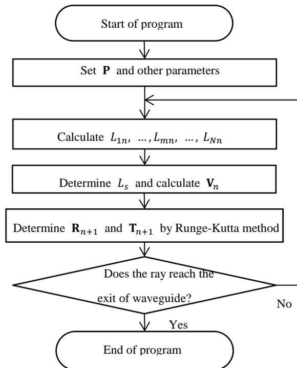
Figure 7-4 Flow chart of the algorithm for ray tracing in an arbitrarily shaped waveguide.
