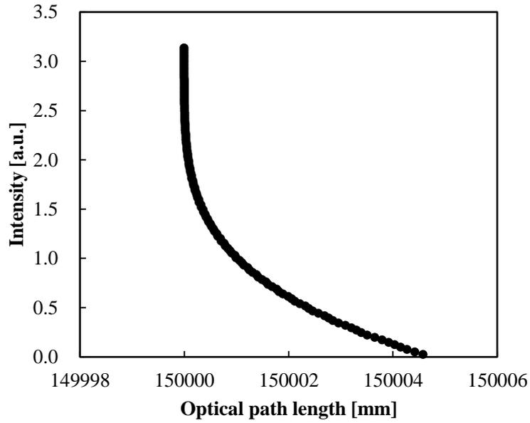
Figure 3-21 Optical path length and intensity of light (refractive index distribution was defined as two-terms and  $n_{\text{cladding}} = 1.000$ ).
