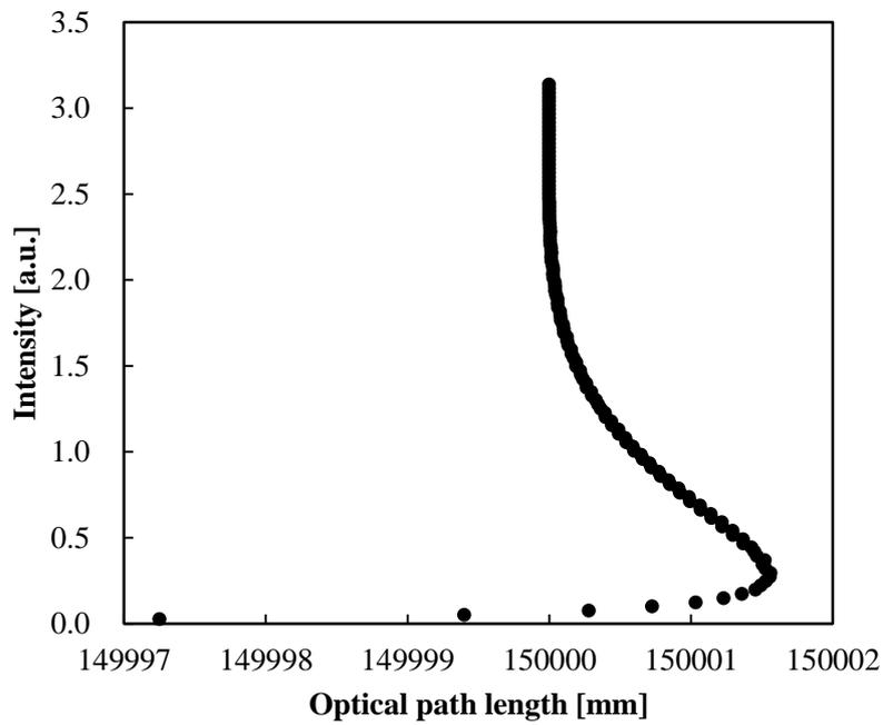
Figure 3-22 Optical path length and intensity of light (refractive index distribution was defined as two-terms and  $n_{\text{cladding}} = 1.485$ ).
