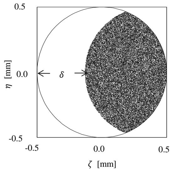
Figure 4-2 The region of the starting position of ray that pass the waveguide without penetrating cladding by Monte Carlo method. Circle indicate the cross-section of  $R_0$ .
