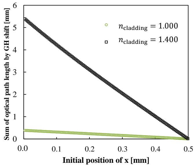
Figure 3-17 Sum of optical path length by GH shift in each initial position of x with different  $n_{\text{cladding}}$  ( $n_{\text{cladding}} = 1.000, 1.400$ ).
