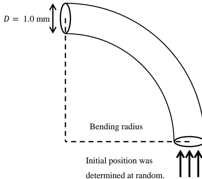
Figure 4-4 Model of bending loss simulation.
