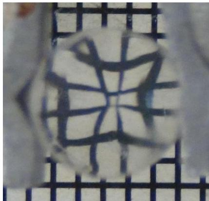
Figure 6-6 Photograph of lattice pattern through the obtained preform rod.
