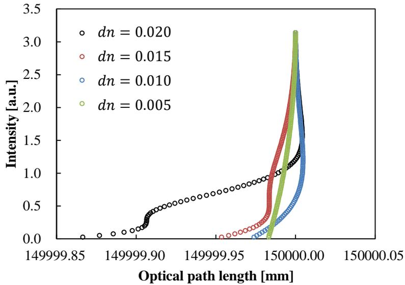
Figure 3-15 The dependence on  $dn$  of optical path length and intensity of light in three-terms refractive index distribution.
