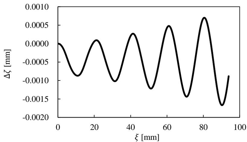
**Figure 7-11** The difference of  $\zeta$  between the calculation of exact ray path and algorithm B with helically exact distribution.
