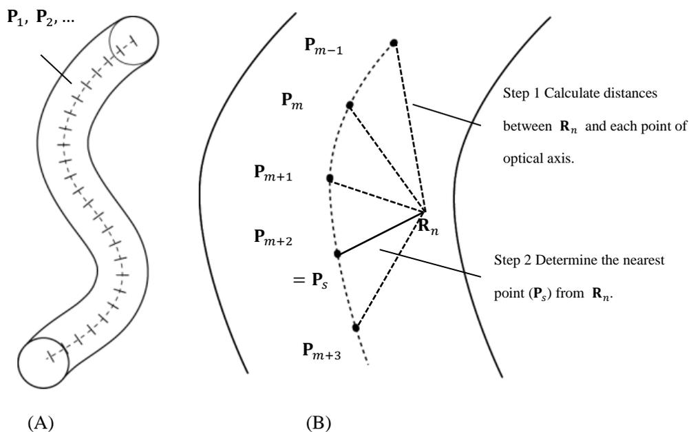
**Figure 7-1 Schematic representation of the ray tracing algorithm for an arbitrarily shaped GI waveguide. (A)  $P$  is a set of points along the optical axis. (B)  $P_s$  is the nearest point on  $P$  from the ray position.**
