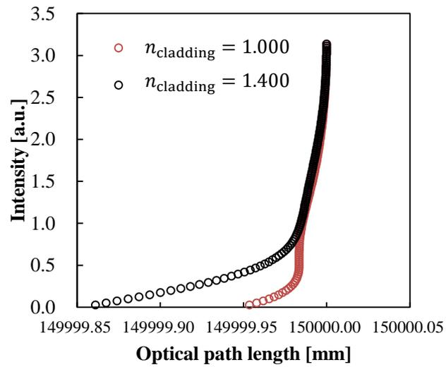
Figure 3-19 Optical path length and intensity of light ( $n_{\text{cladding}} = 1.000, 1.400$ ).
