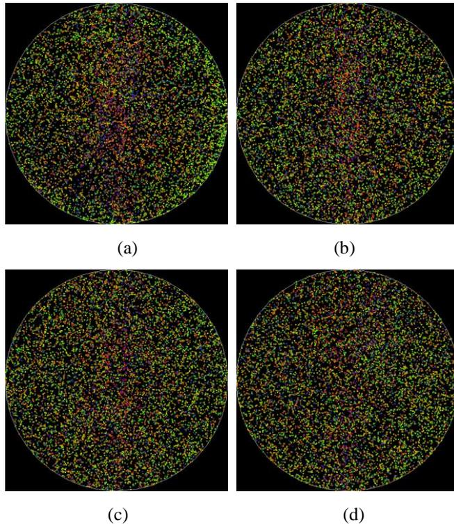
**Figure 7-32** The position of rays on output cross-section of fiber 1 (N-GI waveguide, (a)  $T = 1$ , (b)  $T = 2$ , (c)  $T = 3$ , (d)  $T = 5$ ).
