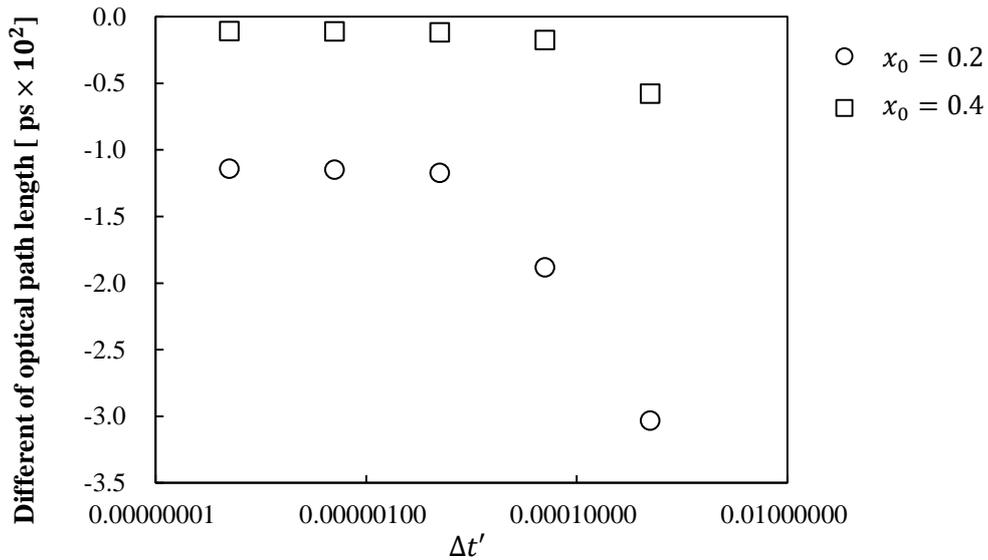
Figure 3-13 Difference of optical path length in each  $\Delta t'$  ( $x_0 = 0.2$  mm,  $0.4$  mm).
