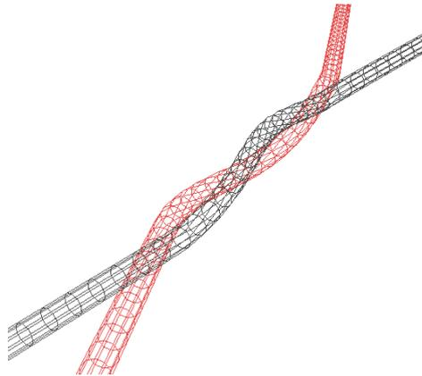
Figure 6-14 Schematic representation of twisting fiber. This figure shows one twisting.
