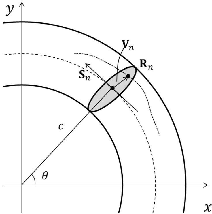
Figure 4-1 Bending waveguide and indication of parameters.
