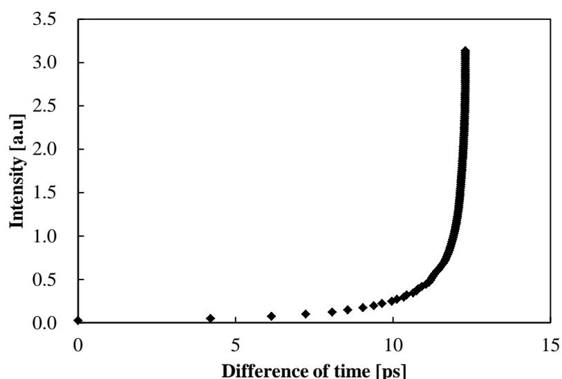
**Figure 3-23 Difference of time of each mode and intensity ( $dn = 0.005$ ,  $n_{\text{cladding}} = 1.495$ ).**
