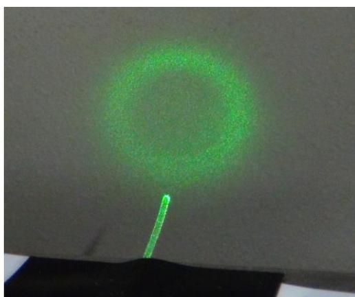
**Figure 6-13 Far field pattern of fabricated N-GI-POF.**
