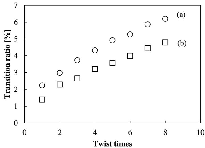
Figure 7-27 Transition ratio of light with  $T$  ( $dn = 0.03$ ,  $g = 2$ ,  $d = 0.03$  mm). (a) Incident light was set in N-GI waveguide. (b) Incident light was set in conventional GI waveguide.
