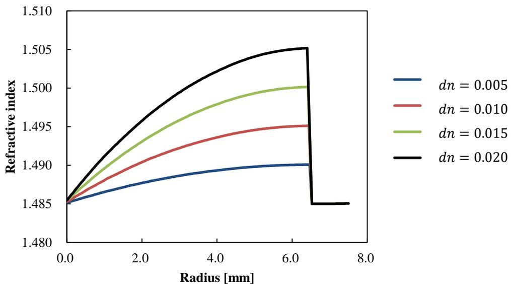
Figure 5-18 Refractive index distribution of each  $dn$ .
