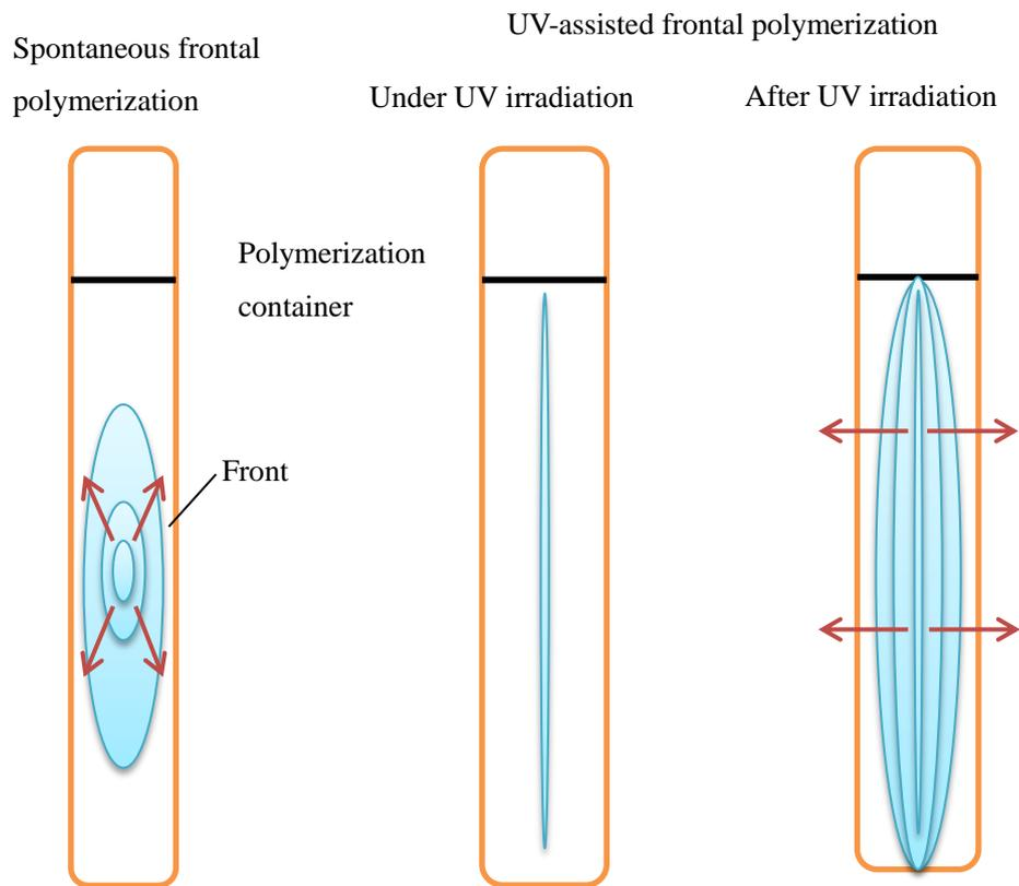
**Figure 6-8** Front expanding of conventional frontal polymerization technique (left) and UV-assisted frontal polymerization technique of UV step (center) and heat step (right).
