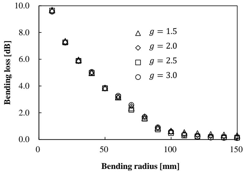
Figure 4-21 Bending loss of refractive index exponent dependence.
