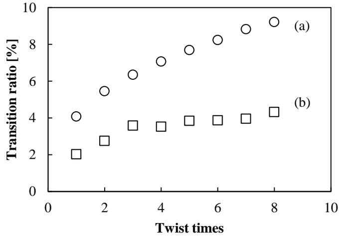
Figure 7-26 Transition ratio of light with  $T$  ( $dn = 0.03$ ,  $g = 4$ ,  $d = 0.03$  mm). (a) Incident light was set in N-GI waveguide. (b) Incident light was set in conventional GI waveguide.
