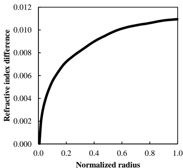
Figure 6-7 The refractive index profile (determined by ray tracing method).
