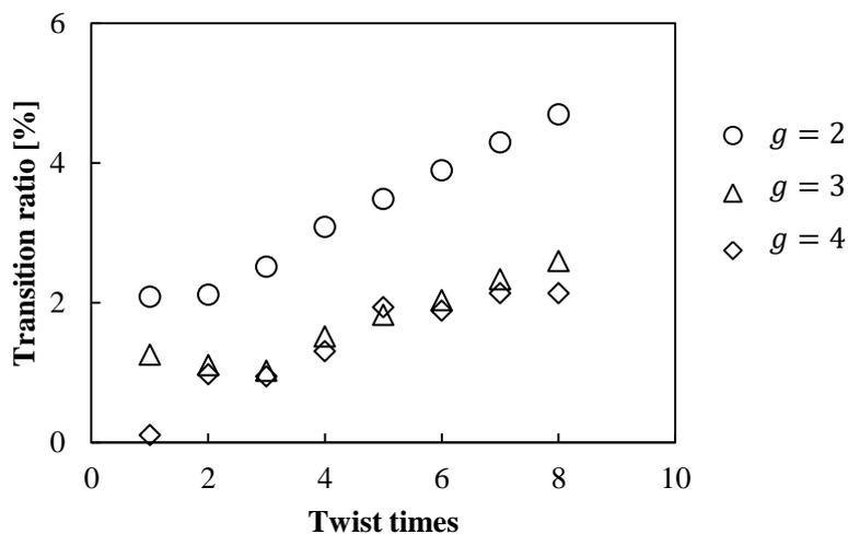
Figure 7-22 Transition ratio of convex GI waveguide with  $T$  ( $g = 2, 3, 4$ ,  $d = 0.03$  mm,  $dn = 0.02$ ).
