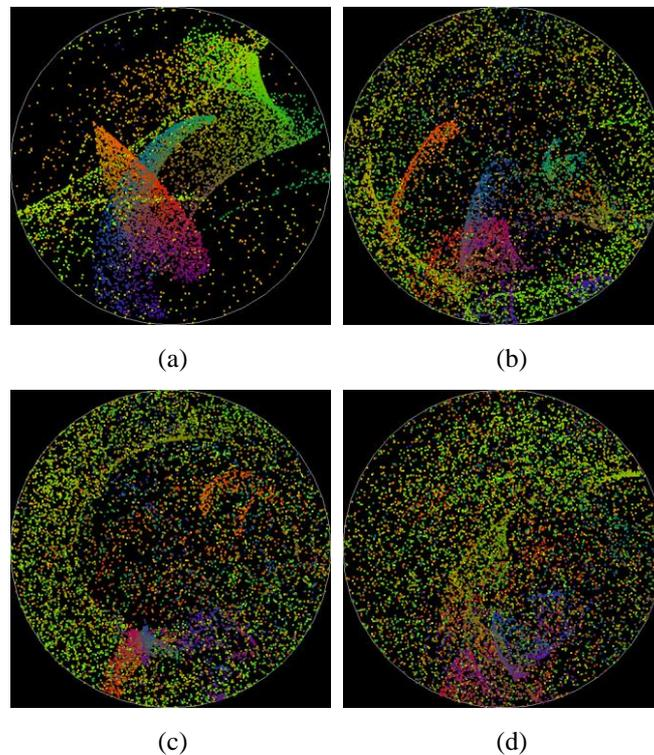
**Figure 7-37** The position of rays on output cross-section of fiber 1 (GI waveguide, (a)  $T = 1$ , (b)  $T = 2$ , (c)  $T = 3$ , (d)  $T = 5$ ).
