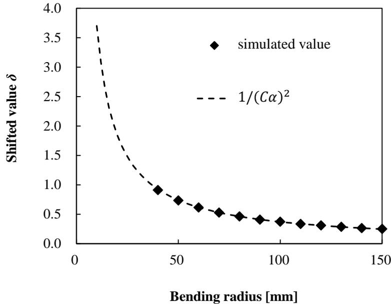
Figure 4-3 Calculated  $\delta$  in each  $C$  (plot) and reported value  $\delta = 1/(C\alpha)^2$  (broken line).
