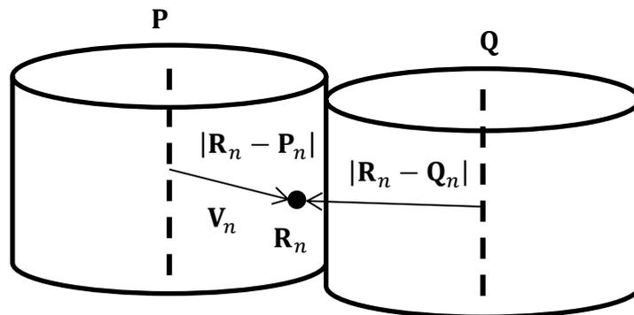
Figure 7-13 Schematic representation of two waveguides in ray tracing.
