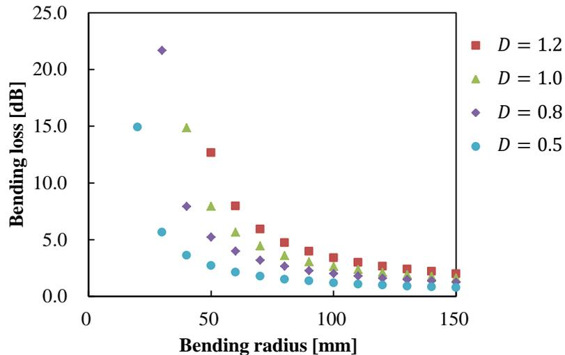
Figure 4-12 Numerical bending loss of in each curvatures about several diameter of waveguide ( $D$  [mm] = 1.2, 1.0, 0.8, 0.5).
