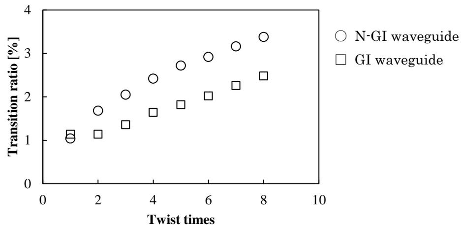
Figure 7-23 Transition ratio of light with  $T$  ( $g = 2$ ,  $d = 0.01$  mm,  $dn = 0.02$ ). Convex GI waveguide and negative GI waveguide is shown.
