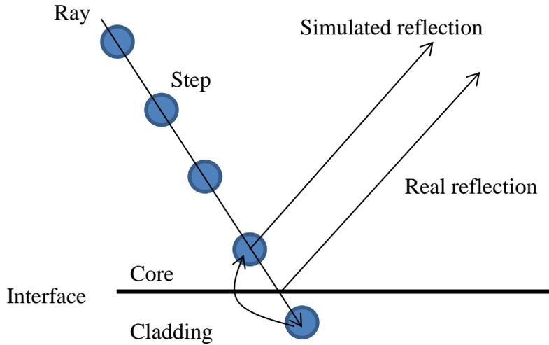
Figure 3-8 Reflection of real phenomenon and ray trace.
