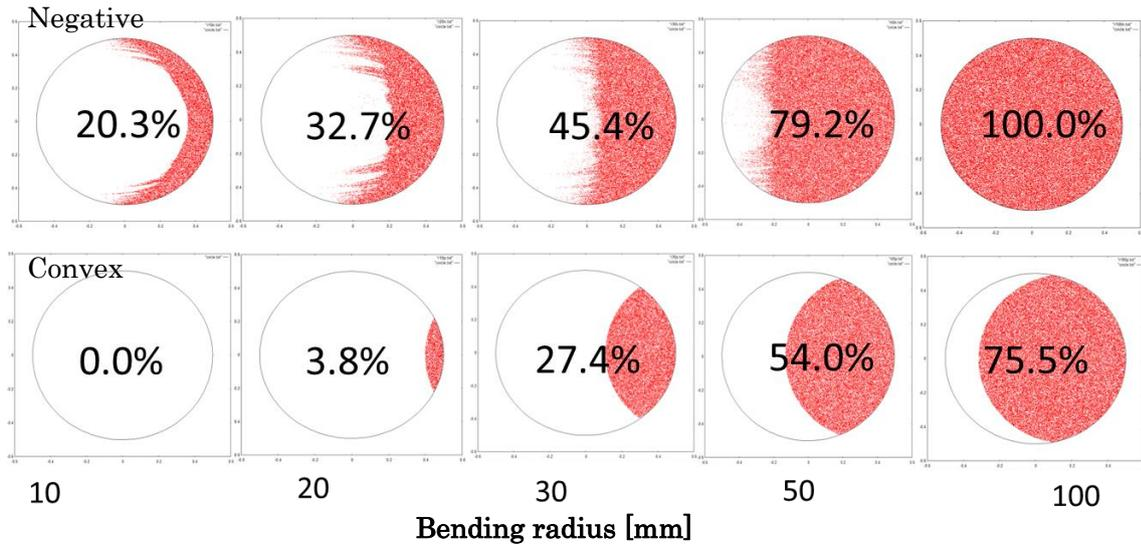
Figure 4-9 Initial position of the ray with passing bending waveguide on cross-section (up: negative, down: positive, 100000 ray, all trial was conducted twice).
