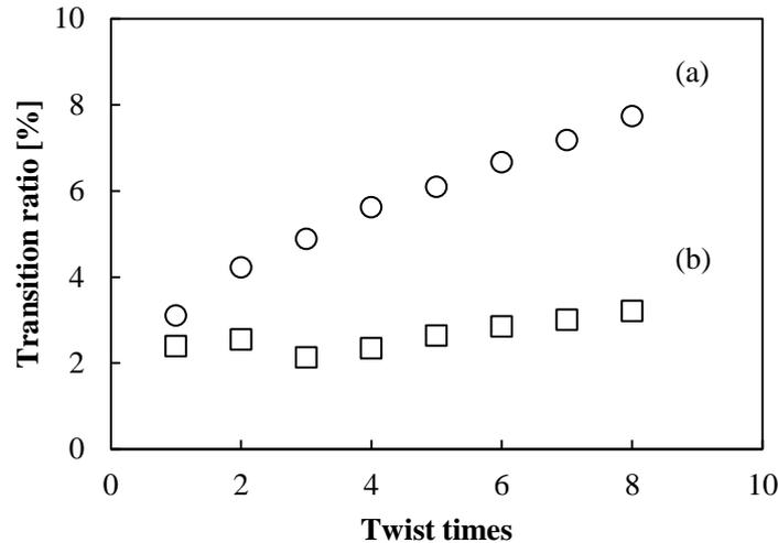
**Figure 7-28** Transition ratio of light with  $T$  ( $dn = 0.01$ ,  $g = 4$ ,  $d = 0.03$  mm). (a) Incident light was set in N-GI waveguide. (b) Incident light was set in conventional GI waveguide.
