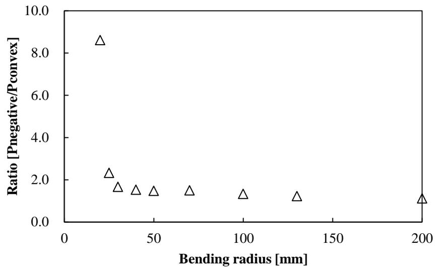
Figure 4-8 The ratio of power of light in negative GI waveguide and convex GI waveguide.
