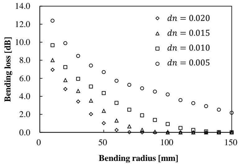
Figure 4-20 Bending loss of refractive index dependence ( $g = 2.0, dn = 0.02, 0.015, 0.010, 0.005$ ).
