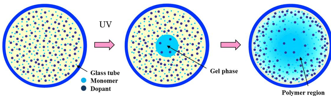
Figure 6-2 UV-assisted frontal polymerization with dopant.
