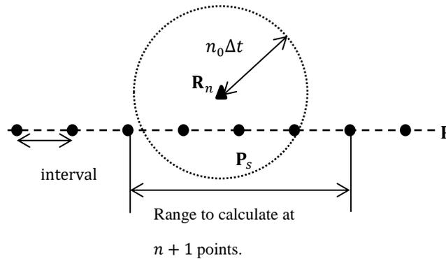
Figure 7-6 Schematic representation of the range to calculate distances between  $R_n$  and  $P$  at  $n + 1$  points.
