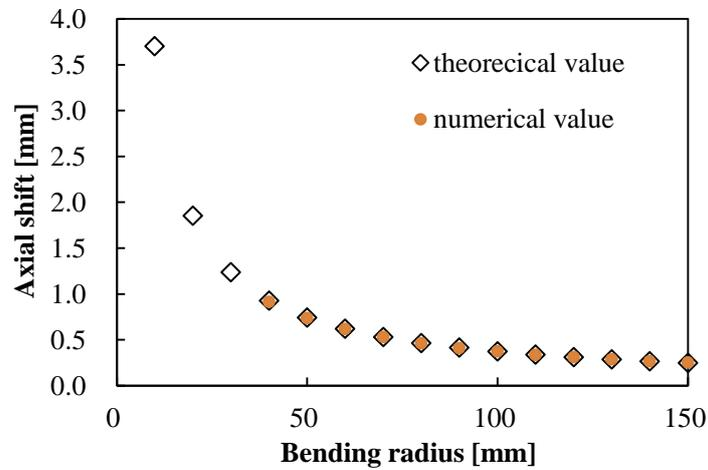
Figure 4-11 Theoretical and numerical axial shift.
