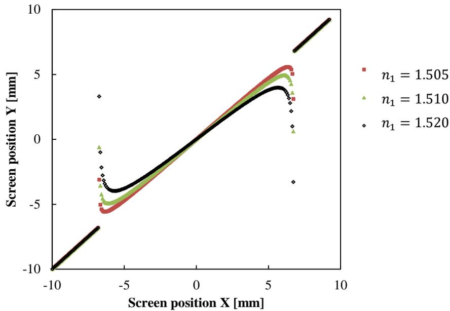
Figure 5-14 Simulated line on the screen through the rod of each refractive index.
