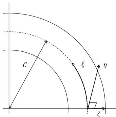
**Figure 7-7 Schematic representation of  $\xi$ ,  $\zeta$ , and  $\eta$ .  $\xi$  is the direction of the optical axis.  $\zeta$  is the direction from the center of curvature to the optical axis.  $\eta$  is the direction perpendicular to the  $\xi - \zeta$  plane.  $C$  is the curvature radius.**
