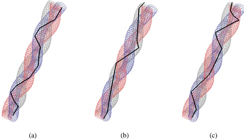
**Figure 7-15 Schematic representation of ray trajectory in triple helix waveguide. (a)Ray propagated to blue fiber. (b)Ray transited to gray fiber. (c) Ray transited to red fiber.**
