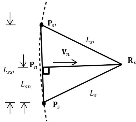
Figure 7-2 Schematic representation of approximation for decreasing error.  $P_s$  is the nearest point from  $R_n$  and  $P_{s'}$  is the next nearest point from  $R_n$ .  $P_n$  is a cross-point of the line  $\overline{P_s P_{s'}}$  ( $L_{SS'}$ ) and a perpendicular line from  $R_n$  to  $L_{SS'}$ .  $V_n$  is the vector from  $P_n$  to  $R_n$ .
