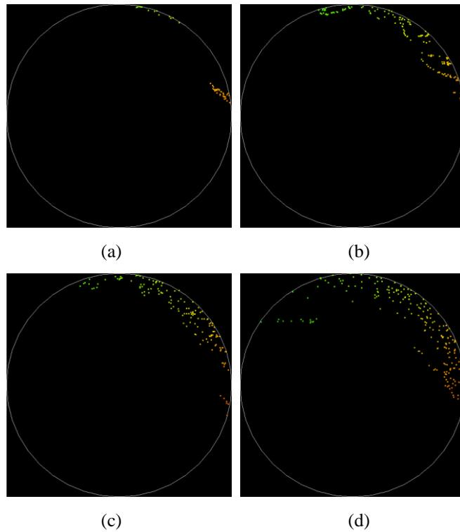
**Figure 7-39** The position of input rays that transferred fiber (GI waveguide, (a)  $T = 1$ , (b)  $T = 2$ , (c)  $T = 3$ , (d)  $T = 5$ ).
