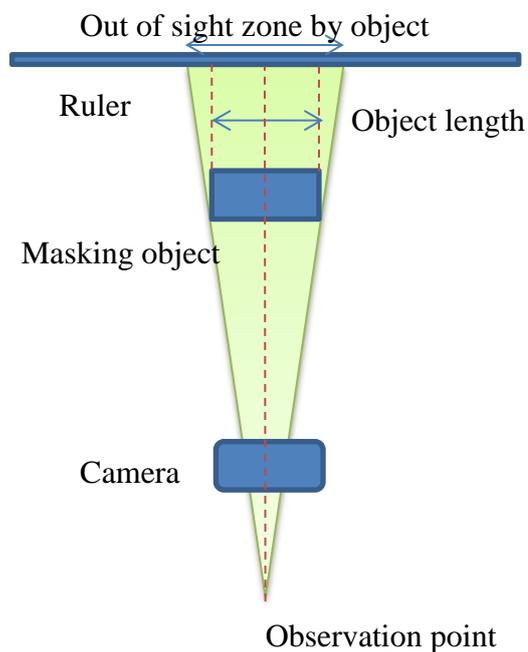
Figure 5-9 Schematic representation of homothetic geometry to determine the observation point.
