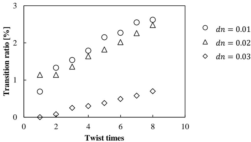
Figure 7-21 Transition ratio of convex GI waveguide with  $T$  ( $g = 2$ ,  $d = 0.01$  mm,  $dn = 0.01, 0.02, 0.03$ ).
