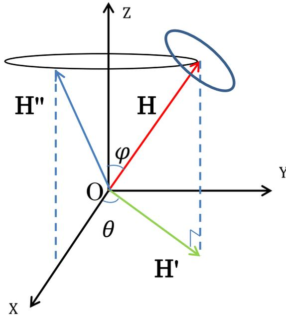
Figure 7-3 Conversion of coordinate from Z axis to optical axis.
