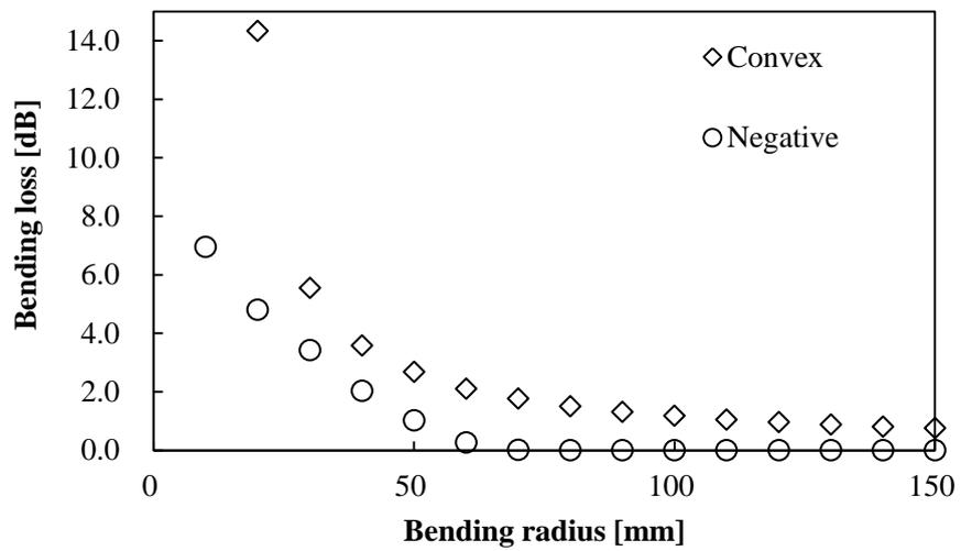
Figure 4-7 Calculated bending loss of convex distribution and negative distribution.
