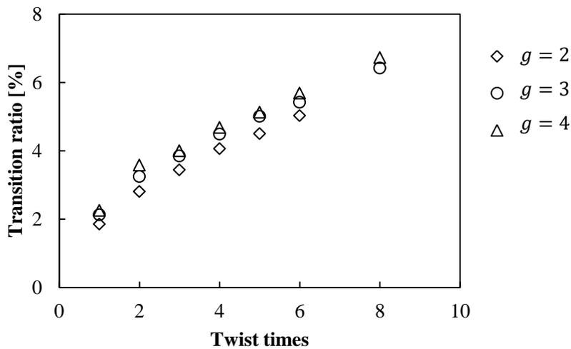
Figure 7-20 Transition ratio of light with  $T$  ( $g = 2, 3, 4, d = 0.03 \text{ mm}, dn = 0.02$ ).
