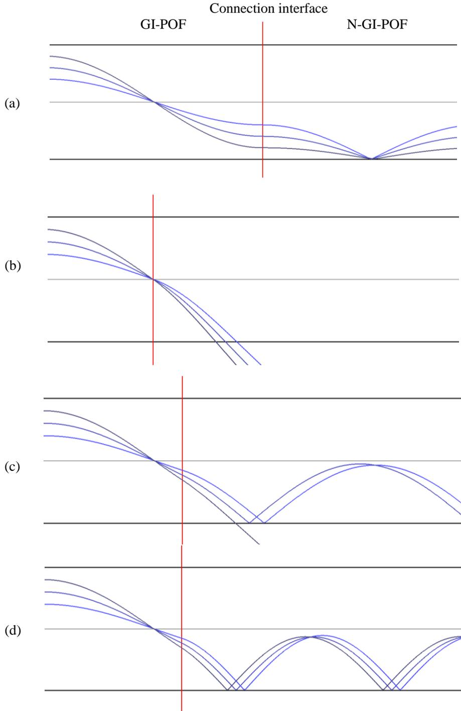
**Figure 2-4 Schematic representation of ray tracing at the GI-POF and N-GI-POF connection. (a) Connection at  $L_p/2$ . (b) Connection at  $L_p/4$ . (c) Connection at  $5L_p/16$ . (d) Connection at  $5L_p/16$  and refractive index difference of N-GI-POF is larger than GI-POF.**
