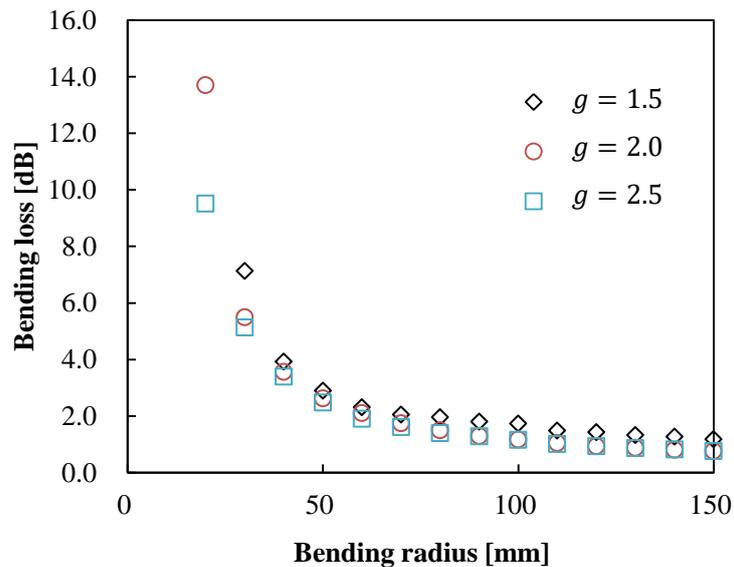
Figure 4-17 Numerical bending loss in each curvatures about different  $g$  ( $g = 1.5, 2.0, 2.5$ ).
