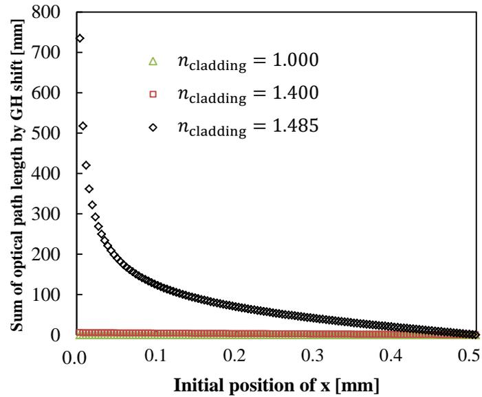
Figure 3-18 Sum of optical path length by GH shift in each initial position of x with different  $n_{\text{cladding}}$  ( $n_{\text{cladding}} = 1.000, 1.400, 1.485$ ).
