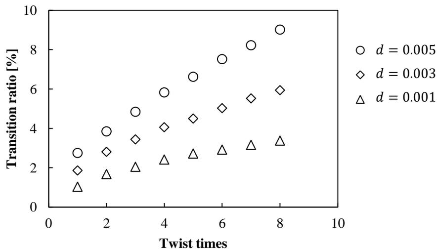
Figure 7-18 Transition ratio of light with  $T$  ( $d$  [mm] = 0.01, 0.03, 0.05,  $g = 2$ ).
