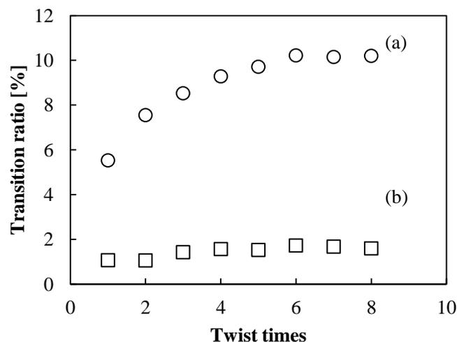
Figure 7-25 Transition ratio of light with  $T$  ( $dn = 0.03$ ,  $g = 6$ ,  $d = 0.03$  mm). (a) Incident light was set in N-GI waveguide. (b) Incident light was set in conventional GI waveguide.
