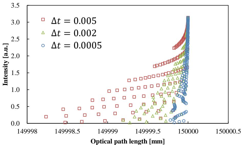
Figure 3-7 Optical path length and Intensity with different  $\Delta t$  in negative type GI waveguide.
