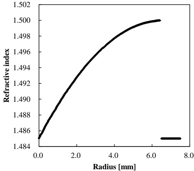
Figure 5-7 Calculated profile from screen data.
