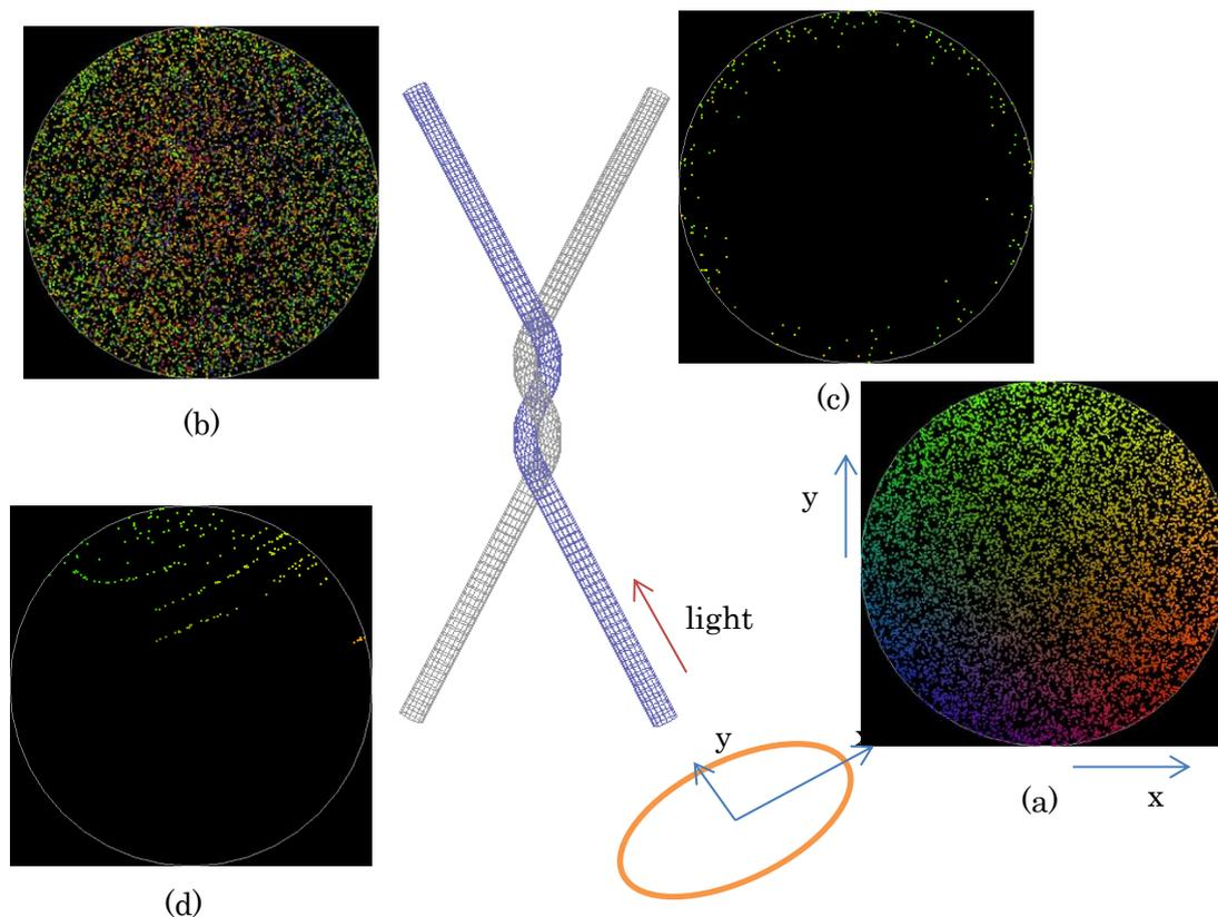
**Figure 7-29 The ray position analysis by ray tracing. Color shows starting ray position of each ray. (a)Starting ray position in fiber1, (b)Output ray position from fiber 1, (c)Output ray position from fiber 2, (d)Corresponding ray to (c) in (a).**
