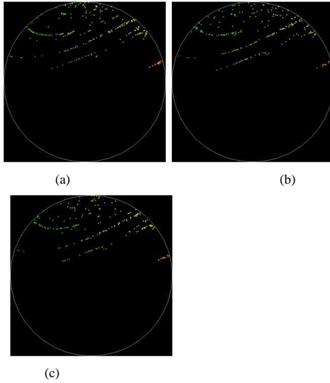
Figure 7-35 The position of input rays that transferred fiber (N-GI waveguide, (a)  $dn = 0.01$ , (b)  $dn = 0.02$ , (c)  $dn = 0.03$ ).
