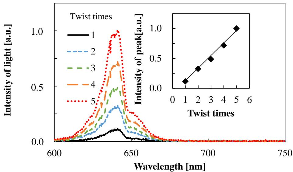
**Figure 6-16** Output light spectra of opposite fiber with twist times. Inset indicates the transition of intensity peaks.
