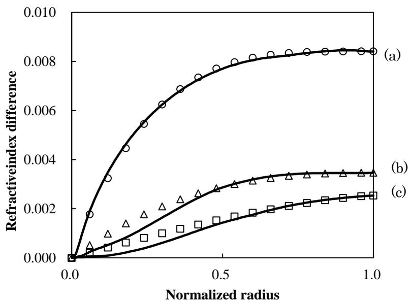
**Figure 6-10 Refractive index profiles (normalized radius and refractive index difference) of obtained preform rod with different pre-polymerization time(a)6.5 h, (b)5.5h, (c)4.5 h). Plot indicates approximated profile((a)  $g = 3.8$ , (b)  $g = 2.6$ , (c)  $g = 1.4$ ).**
