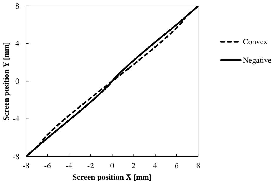
Figure 5-15 Simulated line on the screen through the rod of convex and negative refractive index profile.
