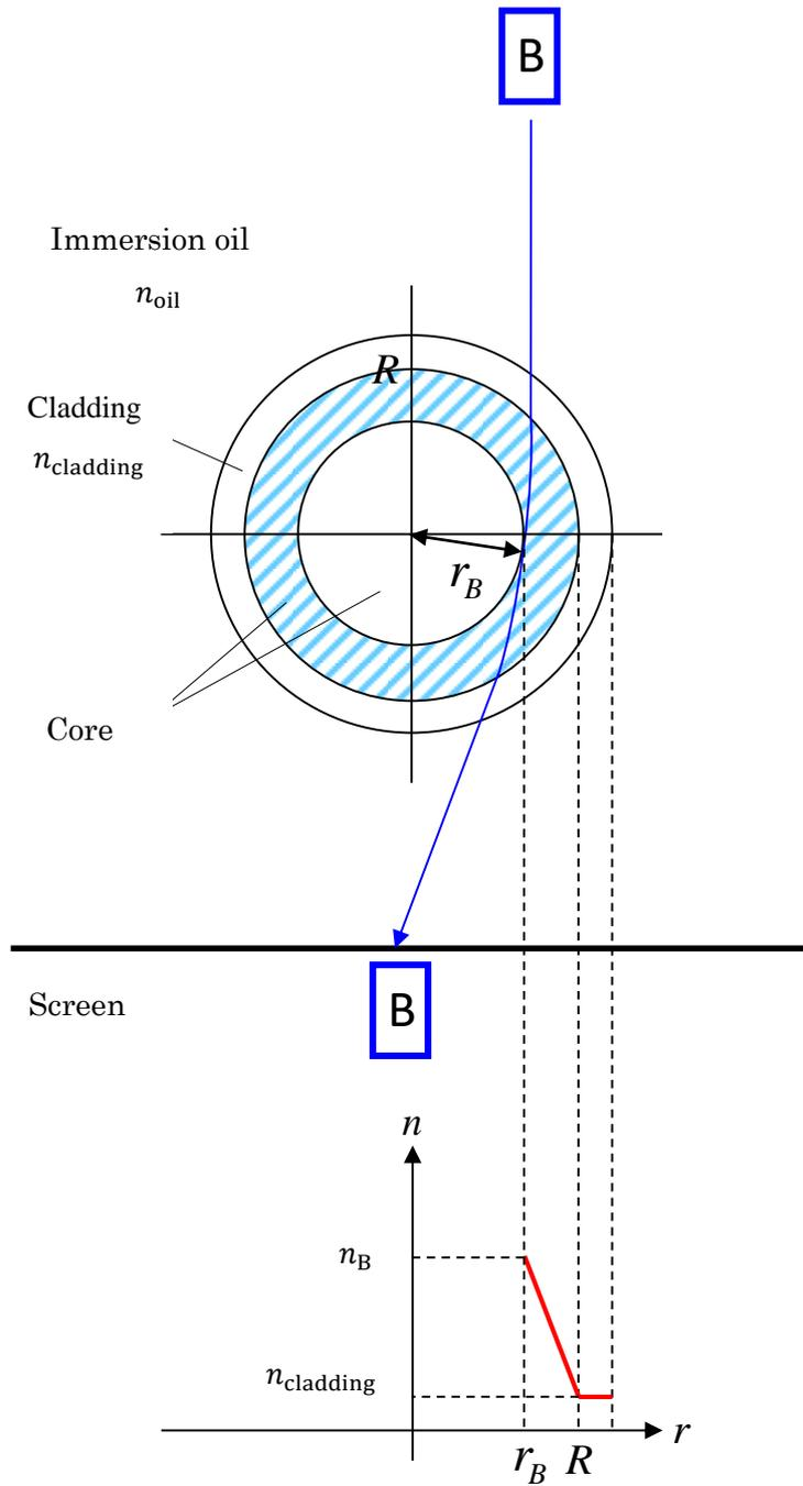
**Figure 5-2 Determination of the refractive index profile by ray B.**
