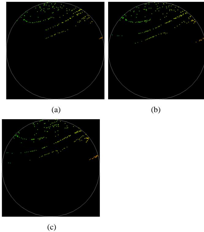
Figure 7-36 The position of input rays that transferred fiber (N-GI waveguide, (a)  $g = 2$ , (b)  $g = 4$ , (c)  $g = 6$ ).
