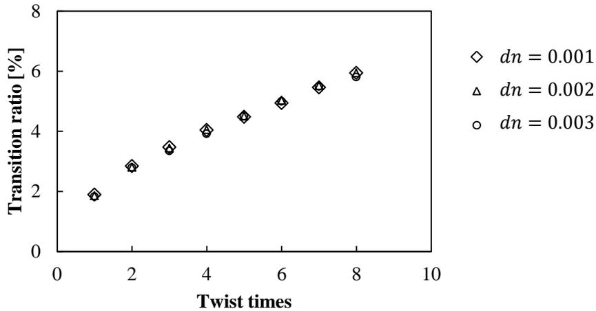
Figure 7-19 Transition ratio of light with  $T$  ( $dn = 0.01, 0.02, 0.03, d = 0.03 \text{ mm}, g = 2$ ).
