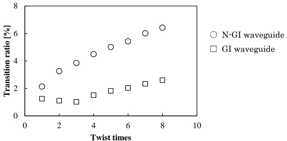
Figure 7-24 Transition ratio of light with  $T$  ( $g = 3$ ,  $d = 0.03$  mm,  $dn = 0.02$ ). Convex GI waveguide and negative GI waveguide is shown.
