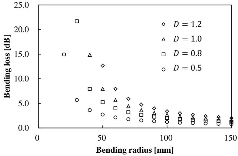
Figure 4-19 Bending loss of diameter dependence ( $dn = 0.01, g = 2.0, D \text{ [mm]} = 1.2, 1.0, 0.8, 0.5$ ).
