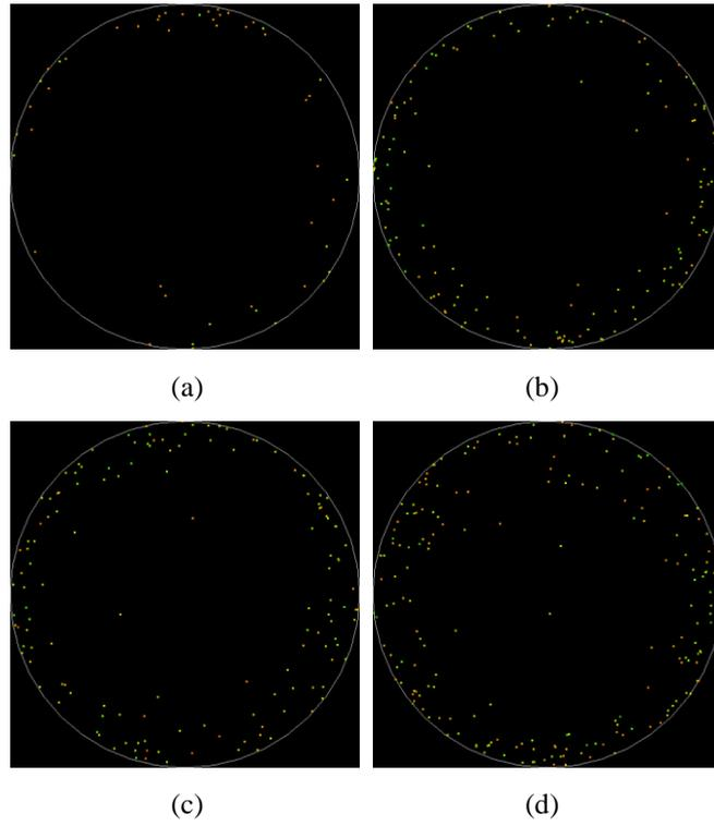
**Figure 7-38** The position of rays on output cross-section of fiber 2 (GI waveguide, (a)  $T = 1$ , (b)  $T = 2$ , (c)  $T = 3$ , (d)  $T = 5$ ).
