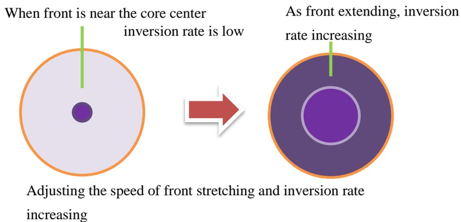
**Figure 6-9** Speed control of front and inversion rate increasing.
