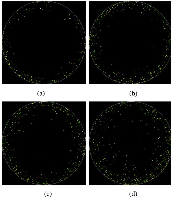
**Figure 7-31** The position of rays on output cross-section of fiber 2 ((a)  $T = 1$ , (b)  $T = 2$ , (c)  $T = 3$ , (d)  $T = 5$ ).
