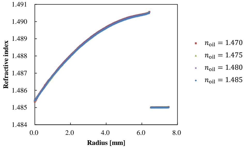
Figure 5-17 Refractive index distribution of each mismatching of immersion oil.
