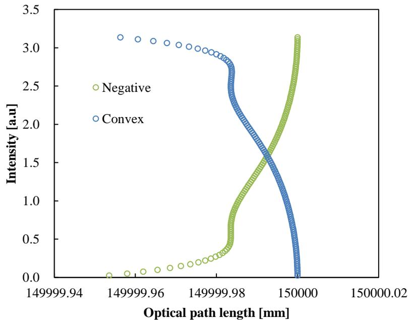
Figure 3-9 Optical path length of each mode and intensity in negative type GI waveguide ( $\Delta t = 0.0005$ ,  $\Delta t' = 5.0 \times 10^{-7}$ ,  $n_{\text{cladding}} = 1.000$ ).
