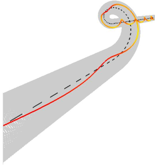
**Figure 7-5 Schematic representation of the ray trajectory using the proposed algorithm. Solid line indicates ray trajectory and broken line indicates optical axis of the waveguide. The waveguide was configured as a straight and helical structure. When trajectory was far from optical axis it shows as yellow.**
