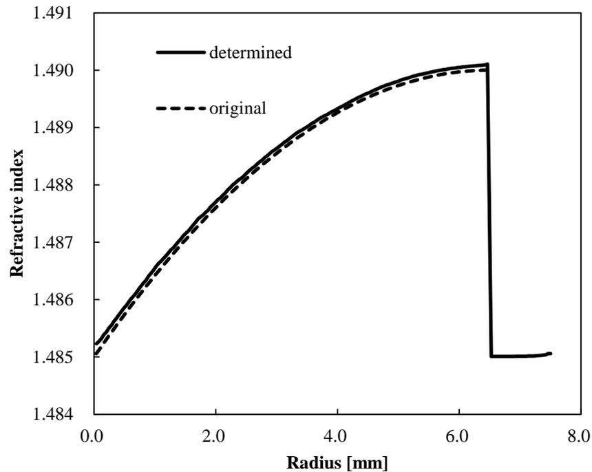
Figure 5-16 Calculated and original profiles of refractive index.
