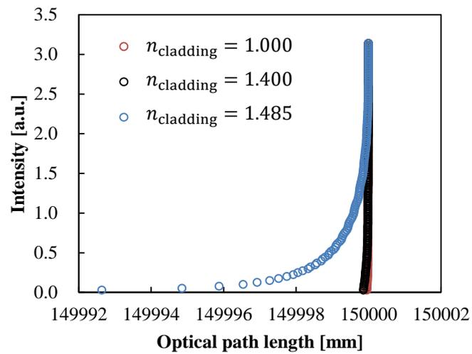
Figure 3-20 Optical path length and intensity of light ( $n_{\text{cladding}} = 1.000, 1.400, 1.485$ ).
