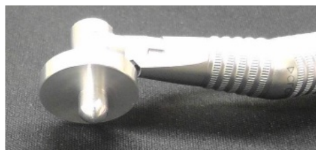
Figure 3.18 Decentering jig used to replace the actual drill when using the simulator
