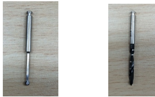
Figure 3.28 Round bur (left) and drill (right) that was used in the experiment
