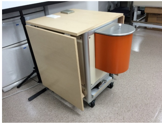
(a) The compact version of the simulator. The legs of the table can be attached and detached to fold the table for mobility.
