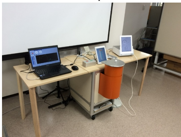
(c) View of the simulator after it is set up. The force-sensible device (orange part of the machine) can be adjusted according to the user height
