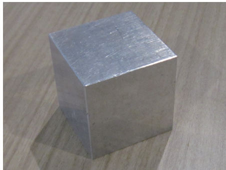
Fig. 2-19: Aluminum block used for through variable control of thermal system.
