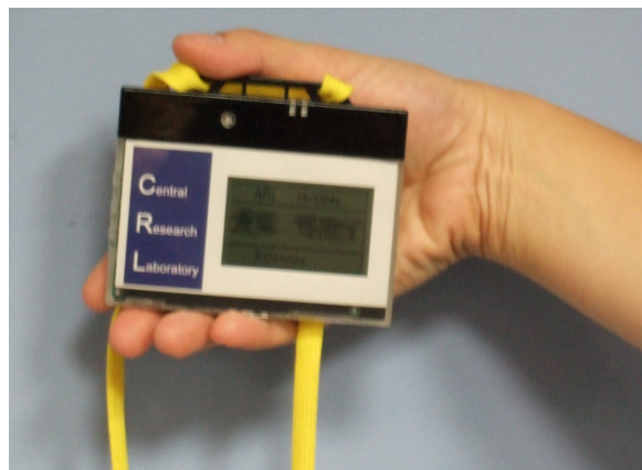
Figure 1.3 Our Wearable Sensor Node Embedded Sound, Acceleration, IR Sensor in Size of Worker's ID Card (3.86 inch × 2.87 inch × 0.35 inch).
