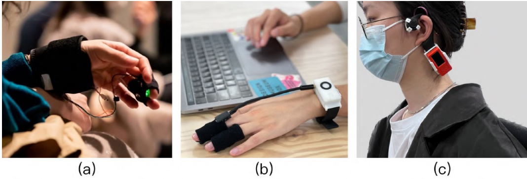
Figure 3.3 Sensing devices used for data collection and recording in this dissertation. (a) and (b) were wrist-worn sensing devices while (c) was ear-based device.
