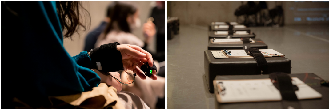
Figure 4.14 Wristband with electrodermal, heart activity, acceleration and gyro sensors. Wristbands and consent from on the seats.
