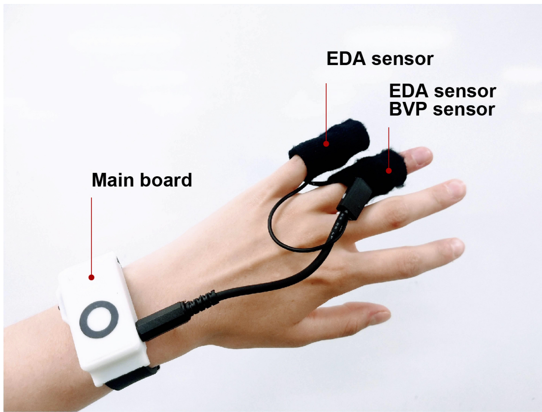
Figure 4.11 Prototype of Smart wristband: The second version of smart wristband with motion sensor, EDA electrodes and BVP sensors on the fingers.
