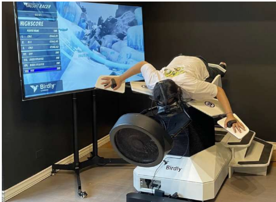
Figure 2.3 Birdly, an immersive flight simulator that mimics avian motion through VR and full-body actuation. (Image source: Birdly VR by Somniacs, used under fair use for academic commentary)
