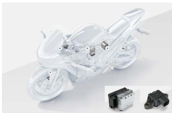
図 1.9 Bosch Motorcycle Stability Control (MSC)
