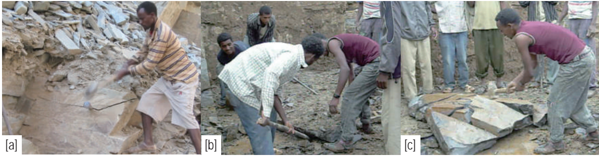
Fig.3-44 Workflow at quarry (a: Driving binito into the rock by medesha ; b: Splitting the rock by using malakino ; c: Smashing the stone block into pieces by medesha ), photo by author.
