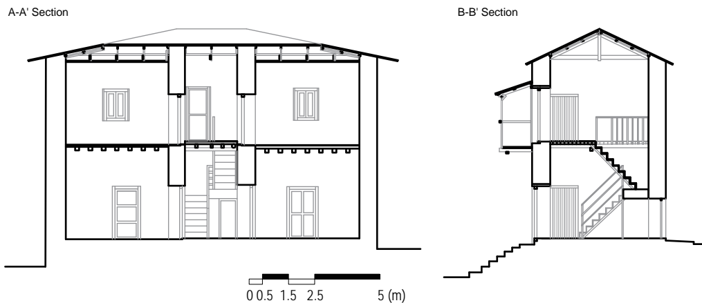
Fig.4-124 Section of an example of a two-story house with symmetric façade (A-A' and B-B' corresponding with Fig.4-71), photo by author.
