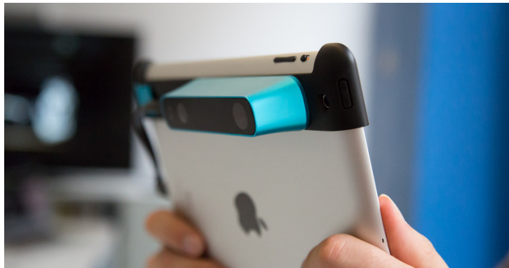
FIGURE C.9: This 3D scanning module is plug on the iPad and allow to scan continuously
