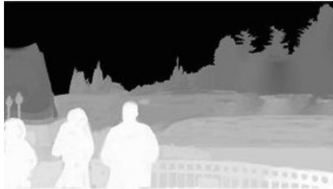
FIGURE C.1: We can see on this depth map various group of pixels with a similar level of grey, they correspond to the various depth plan. When the grey is lighter the plan is closer to the camera.
