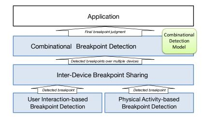
Figure 6.5: Attelia's Multi-Device Hybrid Breakpoint Detection Architecture
