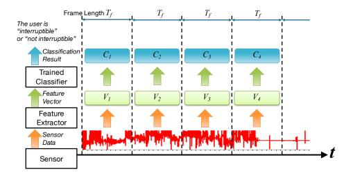
Figure 6.3: Mobile Sensing and Real-Time Detection in Attelia
