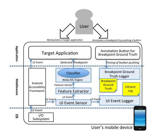
Figure 7.3: System Architecture of Attelia I on Android Platform
