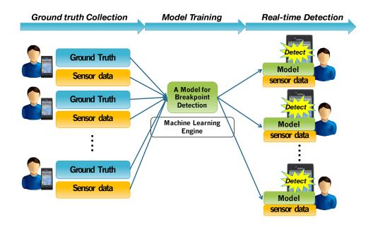
Figure 6.4: Overview of Phases of Machine Learning Technique Attelia Uses
