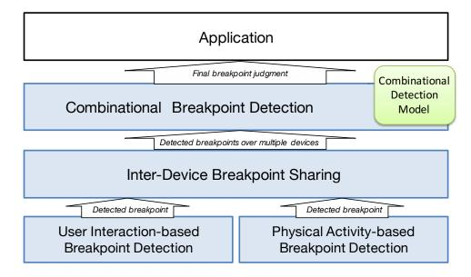
Figure 8.1: Attelia II Layered Breakpoint Detection Architecture
