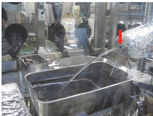
Fig. 5-5 A picture of the molten LiCl-KCl stream from the tube end at 758 K (red arrow indicates the tube end).
