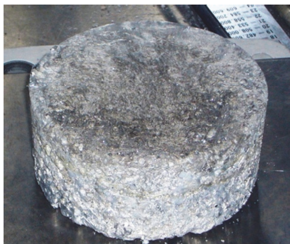
Fig. 5-50 A photograph of Cd–Gd alloy (Gd 0.75 wt%) after removed from the distillation crucible.
