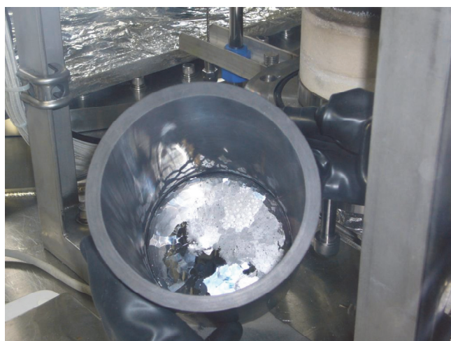
Fig. 5-40 A photograph of the graphite distillation crucible after receiving liquid Cd (Run CC-G17).
