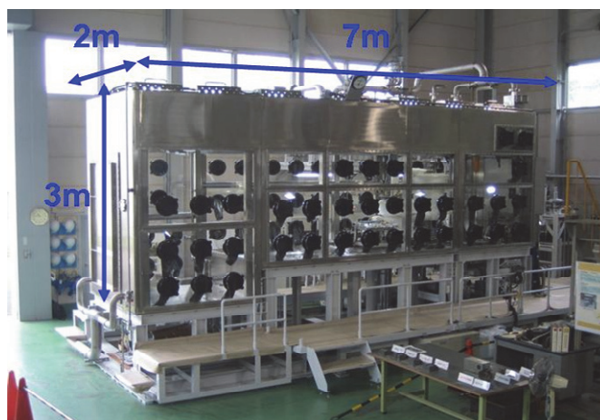
Fig. 5-3 A big-scaled Ar glove box [7 by permission].
