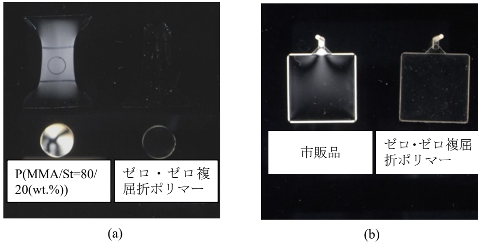
Fig. 3.4 Photographs of polymers between crossed polarizer. (a) Polymer films and bulks of zero zero birefringence polymer and P(MMA/St). (b) Injection molded samples of zero zero birefringence polymer and commercialized polymer.
