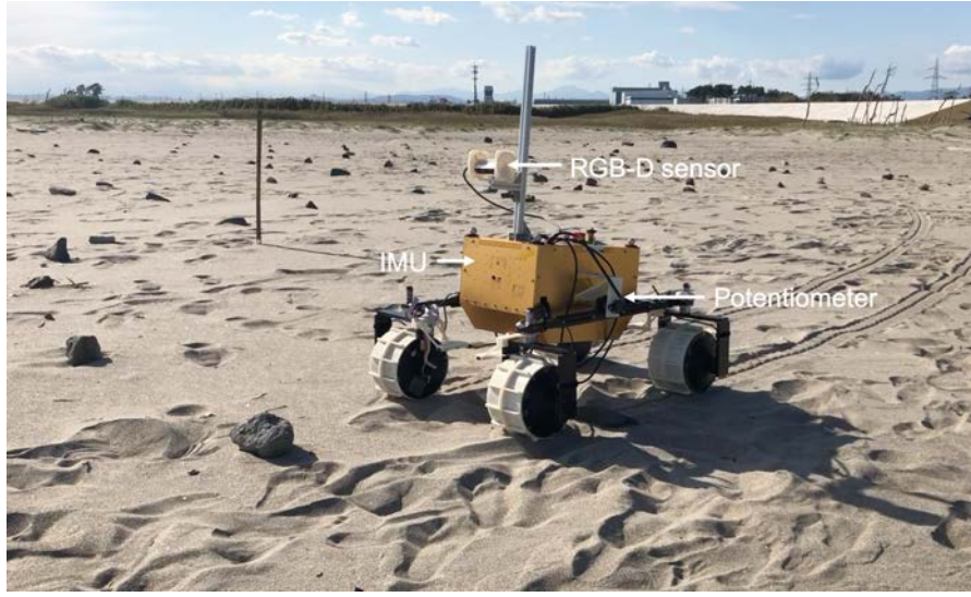
Fig. 2.7: El-Dorado IIB rover testbed on sandy terrain. RGB-D sensor, IMU inside the main body, and potentiometers attached to each side of the body are used for acquiring data.
