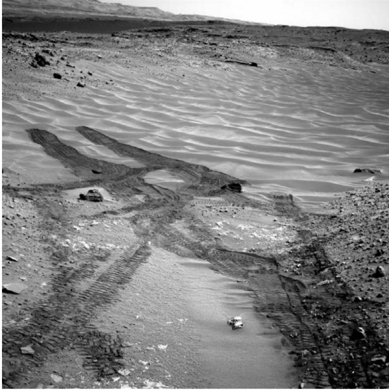
Fig. 2.1: The Hidden Valley on Mars ©NASA/JPL-Caltech. Curiosity experienced excessive wheel slip here and failed to traverse this region although it is relatively flat. At the beginning of the mission, Curiosity was commanded to travel on the flat surface and avoid obstacles such as rocks; however, wheel slip occurred owing to loose sand with megaripples. Wheel traces on these megaripples indicated that Curiosity gave up traversing this surface and turned back to avoid getting stuck.
