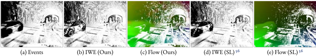
Figure 4.6: DSEC results on the interlaken_00_b test sequence (no GT available). Since GT is missing at IMOs and points outside the LiDAR’s FOV, the supervised method 56 may provide inaccurate predictions around IMOs and road points close to the camera, whereas our method produces sharp edges. For visualization, we use 1M events.
