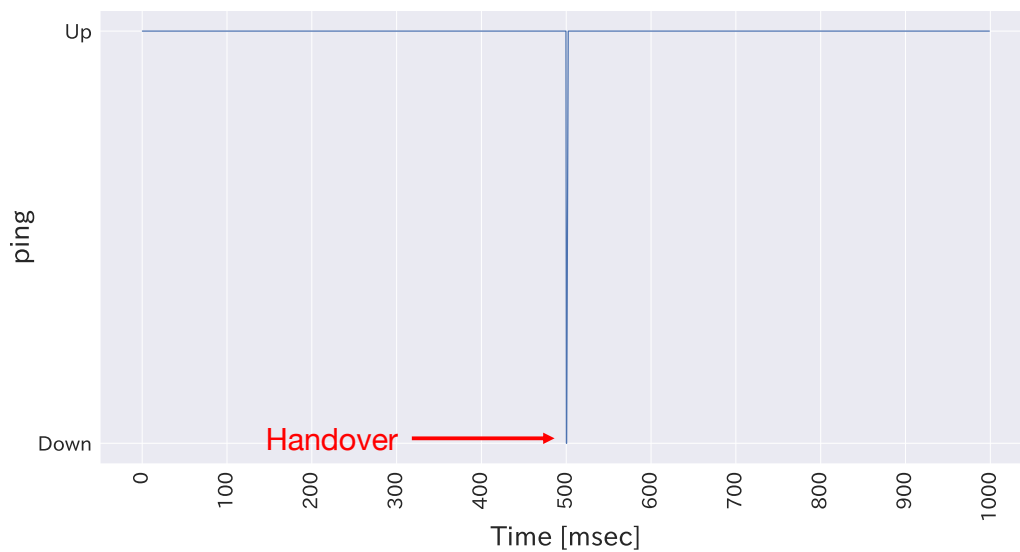
Figure 4.19: Result of ping command for 1 seconds around handover at 40 km/h.
