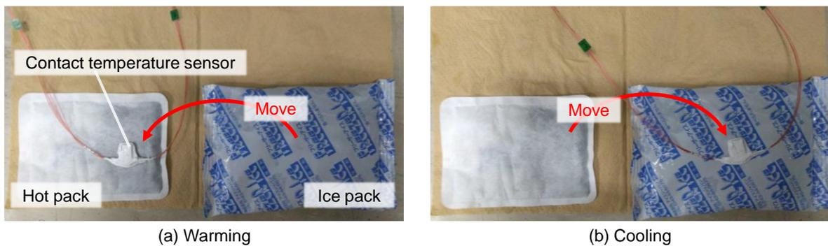
Fig. 2-7 Experimental setup of the control cycle measurement of the temperature analysis environment.
