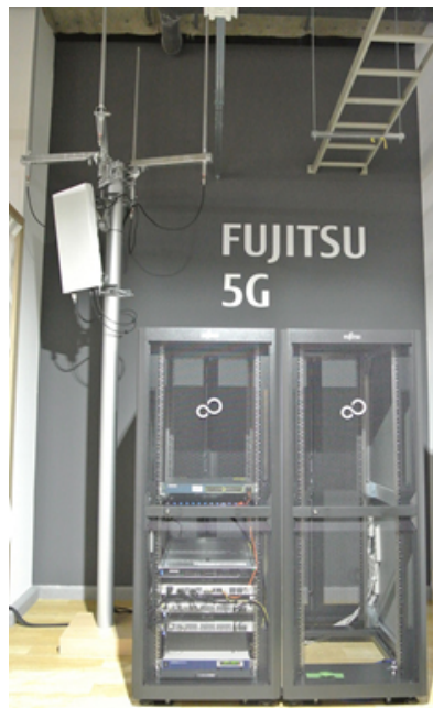
Figure 2.2: Example private 5G base station by Fujitsu [15]
