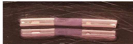
Figure 2.3 Fabrication process of the device (Part 2). (a) A thinner tungsten wire was inserted into the single-layer tube and the collagen pre-gel solution was injected. (b) Plastic jigs were inserted to fix the wire to the center, and the device was incubated to solidify the collagen of the second layer. (c) The tungsten wire was removed to obtain a double-layered collagen tube.
