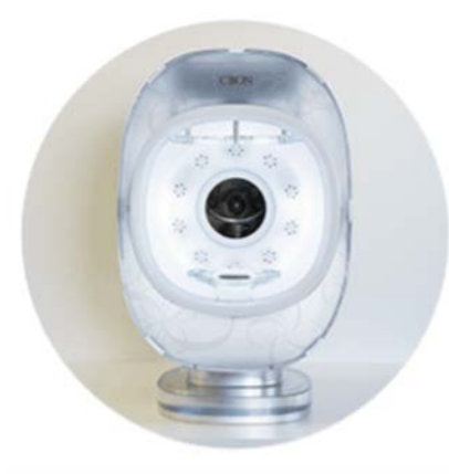
Figure 5.1: The whole facial skin image capture instrument: EPISCAN [4]
