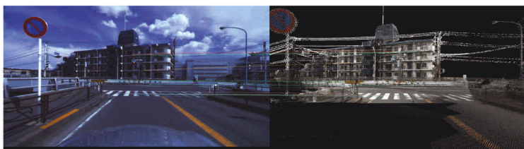
Image matching between vehicle camera image and generated image
