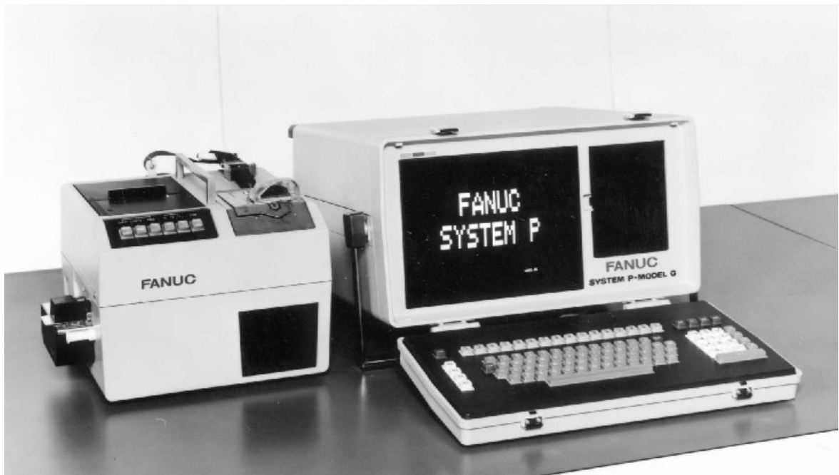
Fig. 2-9 Portable automatic programming system with punched tape reader [34]
