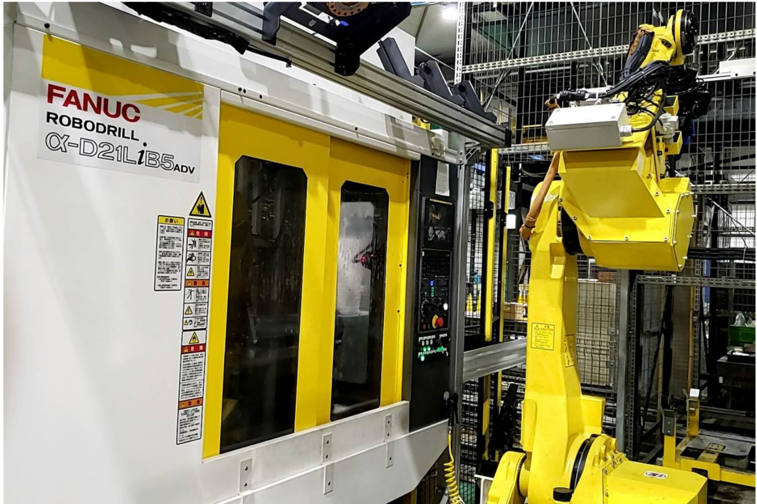
Fig. 5-1 Metal cutting cell
