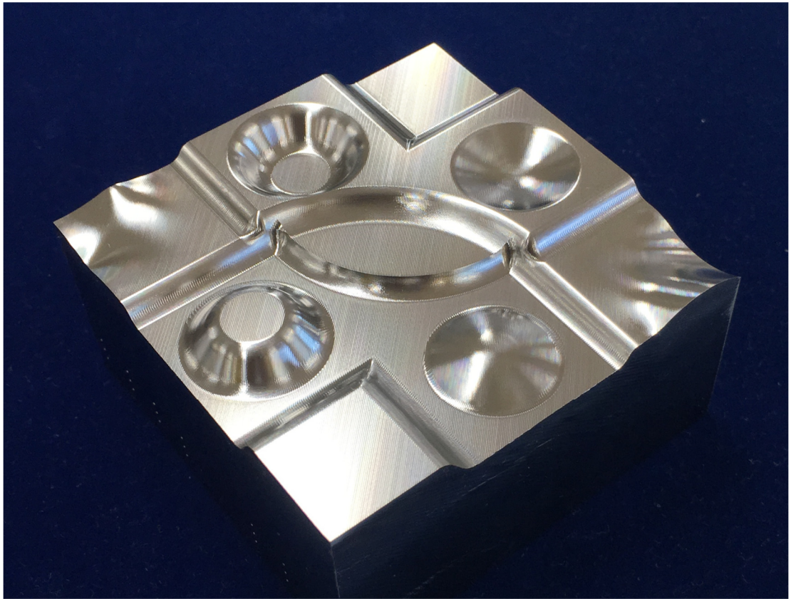
Fig. 4-13 Sample workpiece for freeform machining
