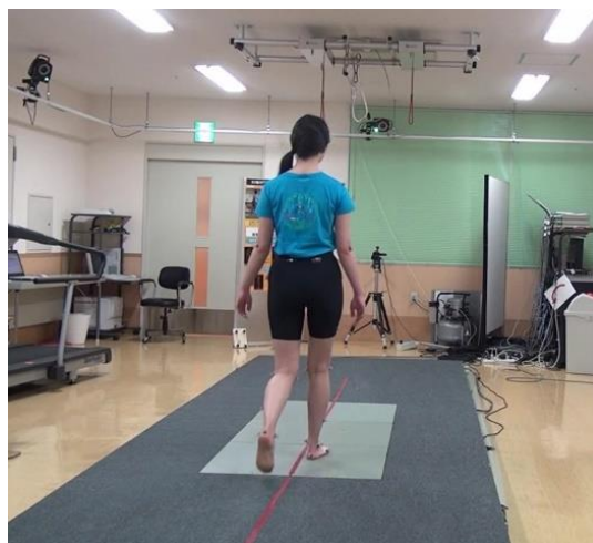
Figure 5.5 The walking experiment for knee joint moment estimation.
