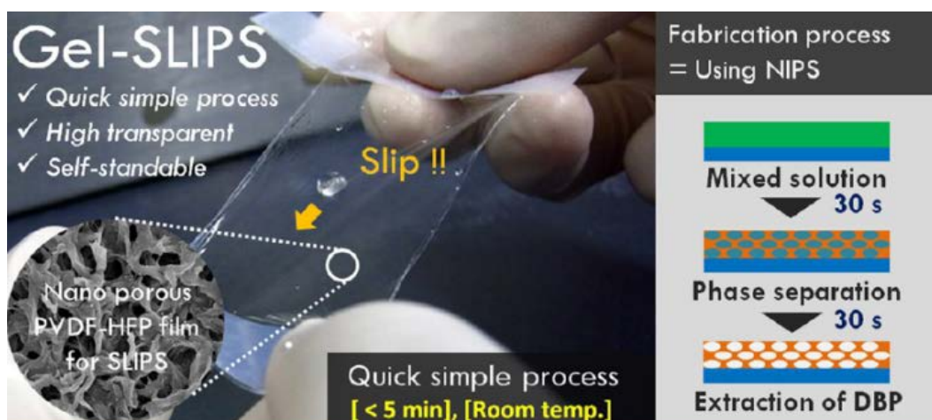
Fig. 3.3. TOC of High-transparency, self-standable Gel-SLIPS fabricated by a facile nanoscale phase separation. Reprinted with permission from ref 12. Copyright 2014 American Chemical Society.
