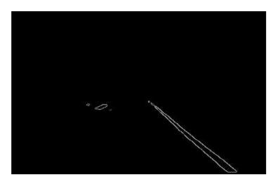
Fig. 2-17: Results of canny edge detection.
