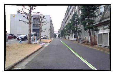
Fig. 2-22: Final result of the line detection.
