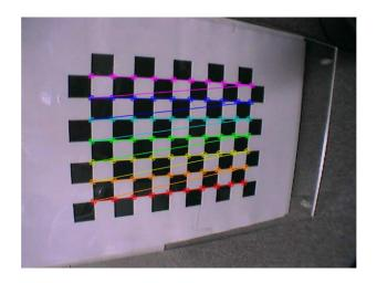
Fig. 2-4: Example of chessboard detection.
