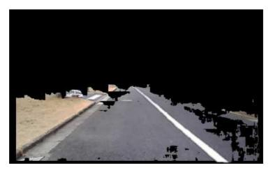
Fig. 2-14: Restriction of the image to the road area.
