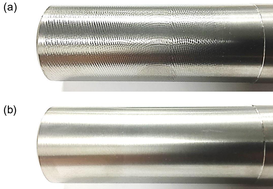
Fig. 6-17 Machined surface of workpiece (a) equal pitch turning (b) unequal pitch turning
