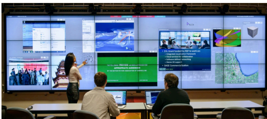
Figure 6.1: A typical SAGE2 session; multiple SAGE2 applications are launched on the Display Clients [2].
