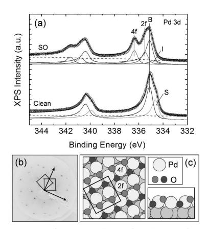
**Figure 4.1.** (a) XP spectra taken from clean metallic and surface oxide (SO) surface. (b) LEED pattern taken from SO/Pd(100) surface. (c) top and side views of model structure of SO formed on Pd(100) surface, where two types of surface Pd atoms are labeled (2f and 4f). Adapted with permission from Ref. P-2. Copyright (2012) American Chemical Society.
