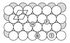
**Figure 1.8.** Possible adsorption sites on a fcc-(111) surface: top (T), bridge (B), hcp-hollow (H) and fcc-hollow (F).
