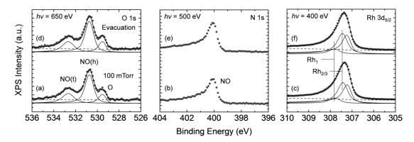
**Figure 3.2.3.** XP spectra from O 1s, N 1s and Rh  $3d_{5/2}$  core levels from a Rh(111) surface taken under 100 mTorr of NO at RT (a, b and c) and after NO gas evacuation and cooled down to 155 K (d, e and f). The photon energies are indicated in each figure. O 1s and Rh  $3d_{5/2}$  spectra were deconvoluted into several components. Adapted with permission from Ref. P-6. Copyright (2015) American Chemical Society.
