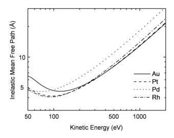
Figure 2.1.3. Simulated inelastic mean free paths for several precious metals.
