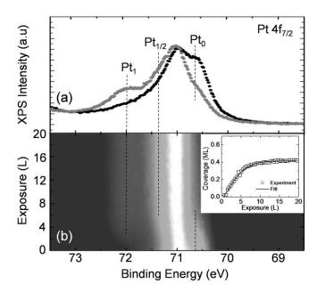
**Figure 3.1.1.** (a) Pt  $4f_{7/2}$  XP spectra taken from CO-free and CO-saturated Pt(111) surfaces. (b) Evolution of Pt  $4f_{7/2}$  level as a function of CO exposure. CO coverage deduced from integrated peak areas (inset).
