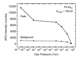
Figure 2.4.3. The pressure dependence of peak and background intensity.
