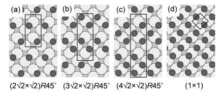
**Figure 3.3.1.** Top views of CO overlayer formed on Pd(100) surface are illustrated (a)  $(2\sqrt{2} \times \sqrt{2})R45^{\circ}$  ( $\theta = 0.50$ ), (b)  $(3\sqrt{2} \times \sqrt{2})R45^{\circ}$  ( $\theta = 0.67$ ), (c)  $(4\sqrt{2} \times \sqrt{2})R45^{\circ}$  ( $\theta = 0.75$ ), and (d)  $(1 \times 1)$ -CO ( $\theta = 1$ ). Large and small balls show the Pd atoms and CO molecules, respectively. The black squares show the unit cells of overlayers.
