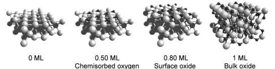
**Figure 1.9.** Evolution of oxygen covered surface depending on the oxygen coverage. Here the metal substrate is modeled by a Pd(100). The small dark and large bright balls indicate O and Pd atoms, respectively. The O surface coverages are estimated in monolayer (ML) scale, with respect to the number of surface Pd atoms.
