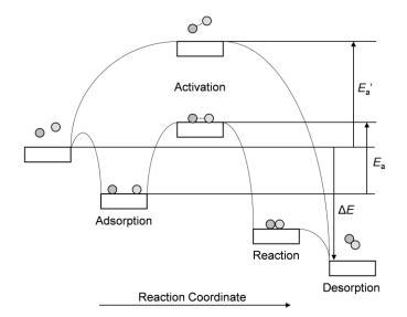
**Figurer 1.1.** The schematic reaction paths with and without catalyst. The  $E_a$  and  $E_a'$  mean the activation energy ( $E_a < E_a'$ ), whereas,  $\Delta E$  means heat of formation. The catalytic reaction is described by a combination of several elementally steps.
