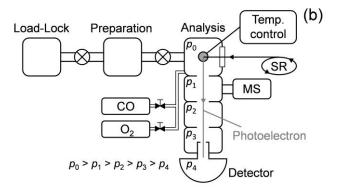
**Figure 2.4.1.** Photographic (a) and schematic (b) images of NAP-XPS system connected to the BL-13A/B at KEK-PF, Japan.
