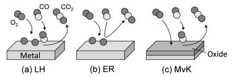
**Figure 1.3.** Reaction mechanisms proposed for CO oxidation reaction. (a) Langmuir-Hinshelwood (LH), (b) Eley-Rideal (ER) and (c) Mars-van Krevelen (MvK).
