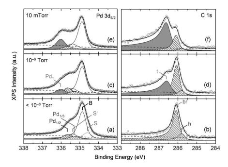
**Figure 3.4.3.** XP spectra for Pd  $3d_{5/2}$  and C 1s levels taken from  $Pd_{70}Au_{30}(111)$  surface at different CO pressures at 298 K. All the XP spectra are shown with curve fitting results, where each component indicates bulk (B), (near) surface (S and S') and CO-bonding Pd (Pdx) in Pd  $3d_{5/2}$  level and CO on hollow (h), bridge (br) and top (t) sites in C 1s level. Adapted with permission from Ref. P-7. Copyright (2015) American Chemical Society.
