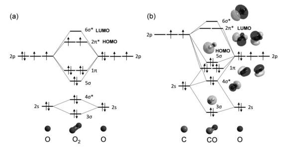
Figure 1.6. Molecular orbitals for diatomic molecules; O<sub>2</sub> (a) and CO (b).
