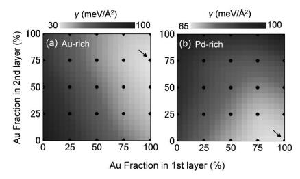
**Figure 3.4.2.** The simulated surface free energies ( $\gamma$ ) of Pd<sub>75</sub>Au<sub>25</sub>(111) on the Au-rich (a) and Pd-rich (b) limit as a function of surface composition. The black dots are the simulated geometries, and the black arrow indicates the most stable surface composition. Adapted with permission from Ref. P-7. Copyright (2015) American Chemical Society.
