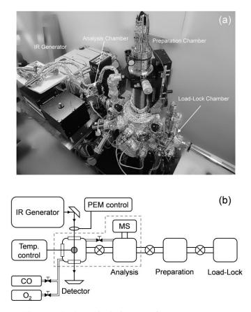
**Figure 2.4.4.** Photographic (a) and schematic (b) images of PM-IRAS system at Yagami campus, Keio University, Japan.
