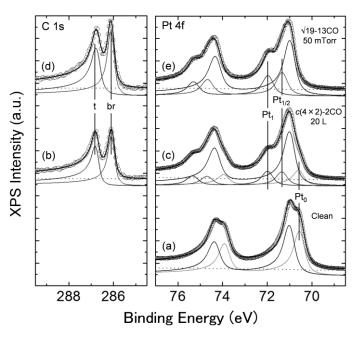
**Figure 3.1.2.** XP spectra Pt 4f and C 1s levels for Pt(111) surface taken under different conditions (clean, 20 L and 50 mTorr) at room temperature. All XP spectra are shown with curve fitting results by  $Pt_0$ ,  $Pt_{1/2}$  and  $Pt_1$  and the bulk component for Pt 4f level and br and t for C 1s level. Assignment of these components is discussed in the main text. Adapted from Ref. P-5 with permission of the PCCP Owner Societies.
