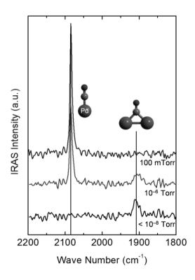
Figure 3.4.5. IRA spectra taken from Pd<sub>70</sub>Au<sub>30</sub>(111) under different CO pressure conditions at 298 K.
