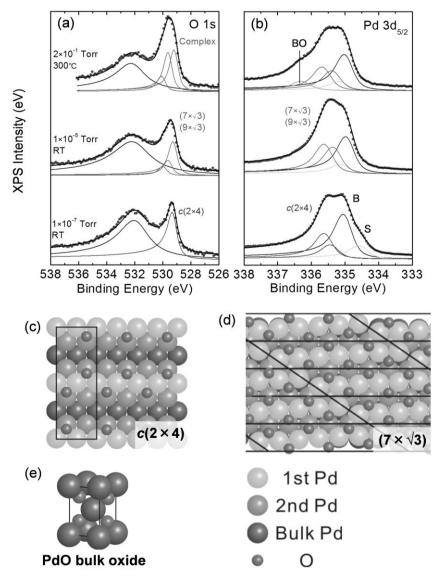
**Figure 4.7.** XP spectra of O 1s (a) and Pd 3d<sub>5/2</sub> (b) levels of the Pd(110) surface taken under various pressure and temperature conditions. The XP spectra are curve fitted into several components. Model structures of chemisorbed oxygen (c and d) and the PdO bulk oxide (BO) (e). Adapted with permission from Ref. P-4. Copyright (2013) American Chemical Society.
