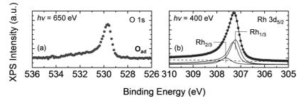
**Figure 3.2.4.** XP spectra from O 1s (a) and Rh  $3d_{5/2}$  (b) levels from an O-adsorbed Rh(111) surface at RT. Irradiated photon energies are indicated in each figure. Adapted with permission from Ref. P-6. Copyright (2015) American Chemical Society.
