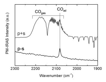
Figure 2.4.5. An example of (PM-)IRA spectrum taken from a CO adsorbed system. The data was taken under 100 mTorr CO ambient.
