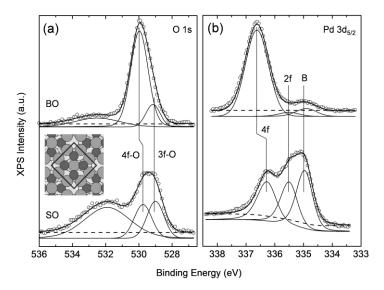
**Figure 4.4.** O 1s (a) and Pd 3d<sub>5/2</sub> (b) XP spectra taken from surface oxide (SO) and bulk oxide (BO) formed on Pd(111) surface. A model structure of the surface oxide is shown in inset. Adapted with permission from Ref. P-1. Copyright (2012) American Chemical Society.
