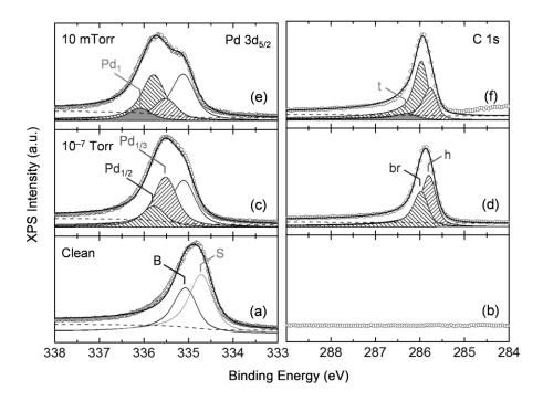
**Figure 3.4.6.** XP spectra for Pd  $3d_{5/2}$  and C 1s levels taken from Pd(111) surface under different pressure condition at 298 K. All XP spectra are shown with curve fitting results, where each component is labelled by B, S and Pd<sub>x</sub> in Pd  $3d_{5/2}$  and h, br and t in C 1s. Adapted with permission from Ref. P-7. Copyright (2015) American Chemical Society.
