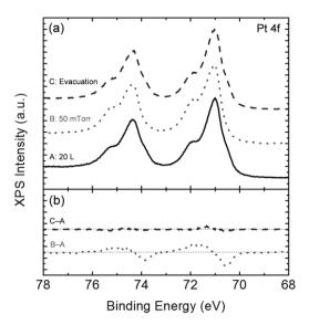
**Figure 3.1.4.** Reversibility for the background pressure of CO overlayer. (a) XP spectra for Pt 4f level taken from a Pt(111) surface under an ultrahigh vacuum (UHV) condition after 20 L CO exposure (A), under 50 mTorr CO (B) and after CO evacuation (C). (b) difference spectra of B and C from A. Adapted from Ref. P-5 with permission of the PCCP Owner Societies.
