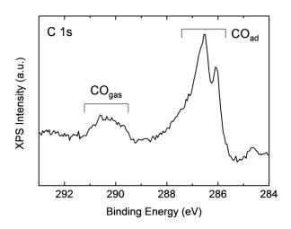
**Figure 2.4.2.** An example of XP spectrum taken from CO adsorbed surface. The data was taken under 10 mTorr CO ambient.
