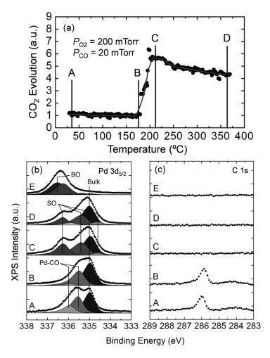
**Figure 4.2** (a) evolution of CO<sub>2</sub> production under exposure to 200 mTorr of O<sub>2</sub> and 20 mTorr of CO. Labels (A, B, C, and D) indicate temperature where XP spectra were recorded. (b, c) XP spectra for  $Pd3d_{5/2}$  and C1s levels taken from Pd(100) surface under the reaction environments. Adapted with permission from Ref. P-2. Copyright (2012) American Chemical Society.
