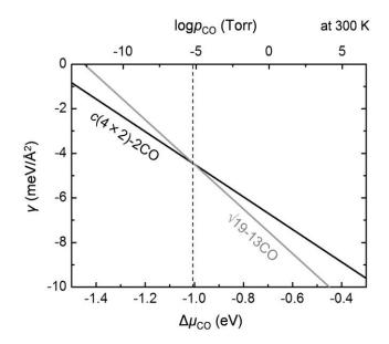
**Figure 3.1.6.** Surface free energies for different CO-induced surface structures formed on Pt(111) as a function of CO chemical potential.
