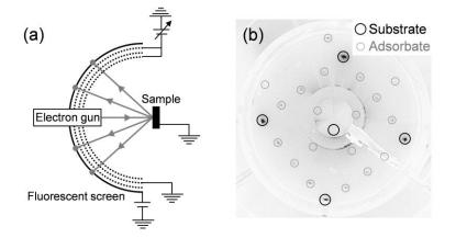
**Figure 2.3.1.** The schematic description of LEED optics (a) and an example of experimentally obtained LEED pattern (CO/Pd(100) surface).
