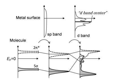
Figure 1.7. Schematic description of molecule-surface interaction.
