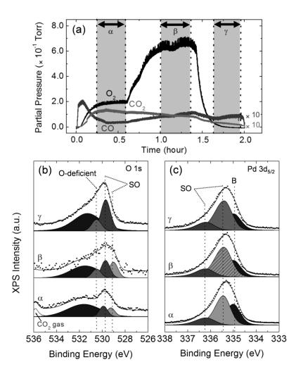
**Figure 4.6.** In-situ monitoring of catalytic CO oxidation on Pd(111) surface at 300 °C. Evolution of O<sub>2</sub>, CO, and CO<sub>2</sub> gases (a), and corresponding XP spectra for O 1s (b) and Pd  $3d_{5/2}$  (c). Adapted with permission from Ref. P-1. Copyright (2012) American Chemical Society.
