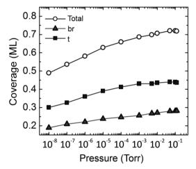
**Figure 3.1.3.** Pressure dependence of the surface CO coverages deduced from Pt  $4f_{7/2}$  level. The fractional coverages of CO on bridge (br) and top (t) are shown by triangle and square plots, respectively, and the total coverage (circle) is a sum of them. Adapted from Ref. P-5 with permission of the PCCP Owner Societies.
