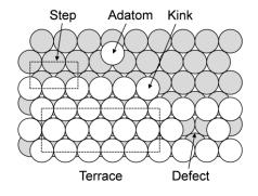
Figure 1.5. Local structures formed on the single crystal surfaces.
