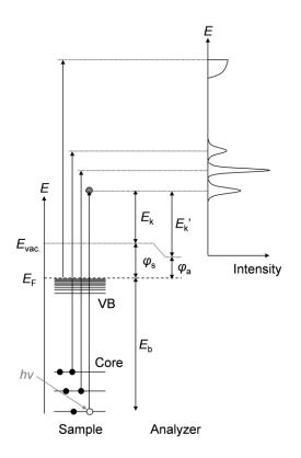
Figure 2.1.1. Schematic description of X-ray induced photoionization process.
