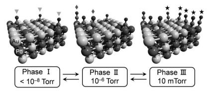
**Figure 3.4.7.** Summary of CO adsorption behavior on  $Pd_{70}Au_{30}(111)$  surface at different CO pressures. Phase I: CO adsorbs on bridge and hollow sites of contiguous dimer and trimer Pds dispersed on the surface. Phase II: CO adsorbs on top site on isolated monomer Pd. Phase III: The COs change adsorption sites from bridge and hollow sites to on top sites of contiguous Pds. Adapted with permission from Ref. P-7. Copyright (2015) American Chemical Society.
