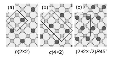
**Figure 3.3.4.** Top views of NO overlayer formed on Pd(100) surface, (a and b)  $p(2 \times 2)$  and  $c(4 \times 2)$  ( $\theta = 0.25$ ), and (c)  $(2\sqrt{2} \times \sqrt{2})R45^{\circ}$  ( $\theta = 0.50$ ). Large and small balls show the Pd atoms and CO molecules, respectively. The black squares show the unit cells of the overlayers. Adapted from Ref. P-3. Copyright (2013), with permission from Elsevier.
