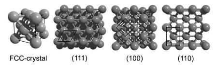
Figure 1.4. The unit cell and the low-index (111), (100) and (110) surfaces for fcc crystal.
