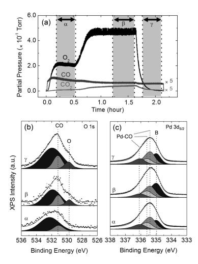
**Figure 4.5.** In-situ monitoring of catalytic CO oxidation on Pd(111) surface at 200 °C. Evolution of  $O_2$ , CO, and  $CO_2$  gases (a), and corresponding XP spectra for O 1s (b) and Pd  $3d_{5/2}$  (c). Adapted with permission from Ref. P-1. Copyright (2012) American Chemical Society.
