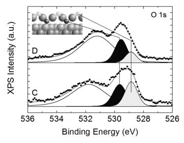
**Figure 4.3.** O1s XP spectra under catalytic conditions taken at point C and D. The CO<sub>2</sub> formation rate decreases from C to D, with increasing the temperature. Model structure of the  $(\sqrt{5} \times \sqrt{5})$ R27° surface oxide formed on Pd(100) is shown in inset. A broad feature at a higher binding energy is a contribution from Pd 3p<sub>3/2</sub>level. Adapted with permission from Ref. P-2. Copyright (2012) American Chemical Society.
