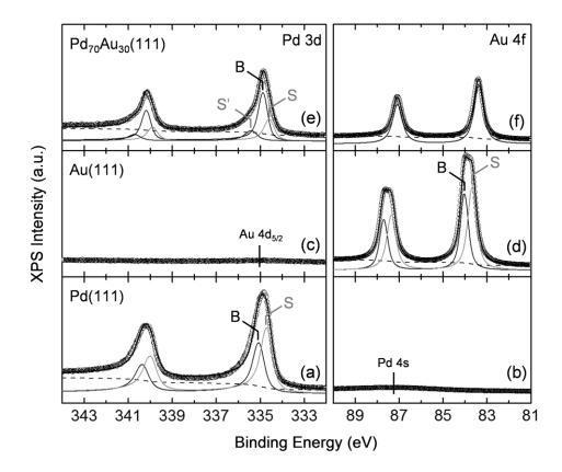
**Figure 3.4.1.** XP spectra for Pd 3d and Au 4f levels taken from CO-free Pd(111), Au(111) and Pd<sub>70</sub>Au<sub>30</sub>(111) surfaces at 298 K. All XP spectra are shown with curve fitting results, where each component indicates the bulk (B) and (near) surface (S and S') metal atoms. Adapted with permission from Ref. P-7. Copyright (2015) American Chemical Society.
