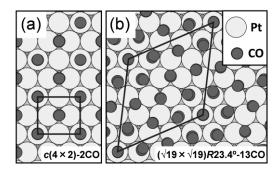
**Figure 3.1.5.** The top views of simulated overlayers of  $c(4 \times 2)$ -2CO (a) and  $\sqrt{19}$ -13CO (b). The black enclosures indicate the unit cells of the structures. Here the surface and molecule are modelled by large and small balls, respectively. Adapted from Ref. P-5 with permission of the PCCP Owner Societies.
