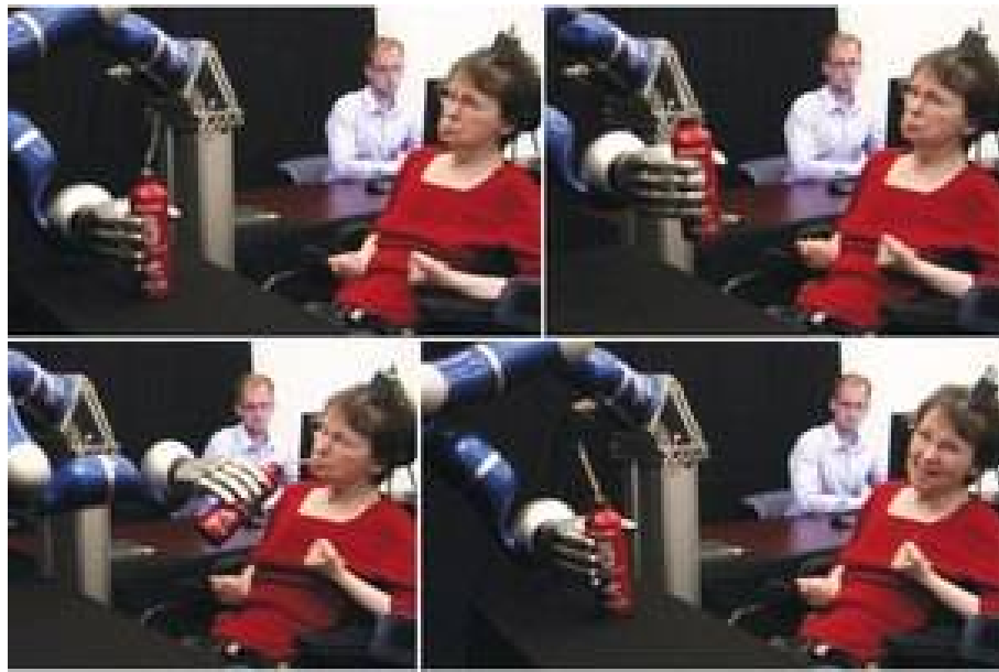
Figure 1.3: The patient with tetraplegia controlling a helping hand robot with her brain waves for the drink bottle. Image courtesy of Hochberg et al. [4].
