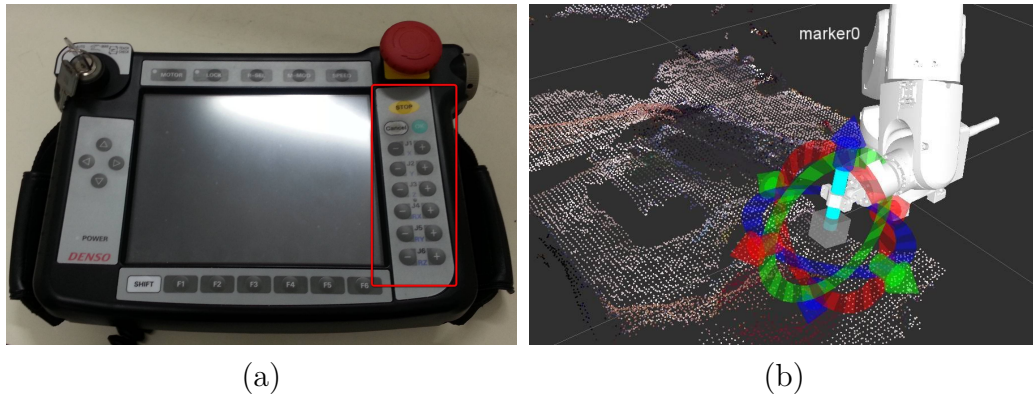
Figure 5.2: (a) The teaching pendant that allows the users to control each joint or axis separately by using the buttons in red rectangle. (b) The interactive marker for controlling the end effector of the robot in ROS (rviz). The arrows and rings are used for translation and orientations controls, respectively.
