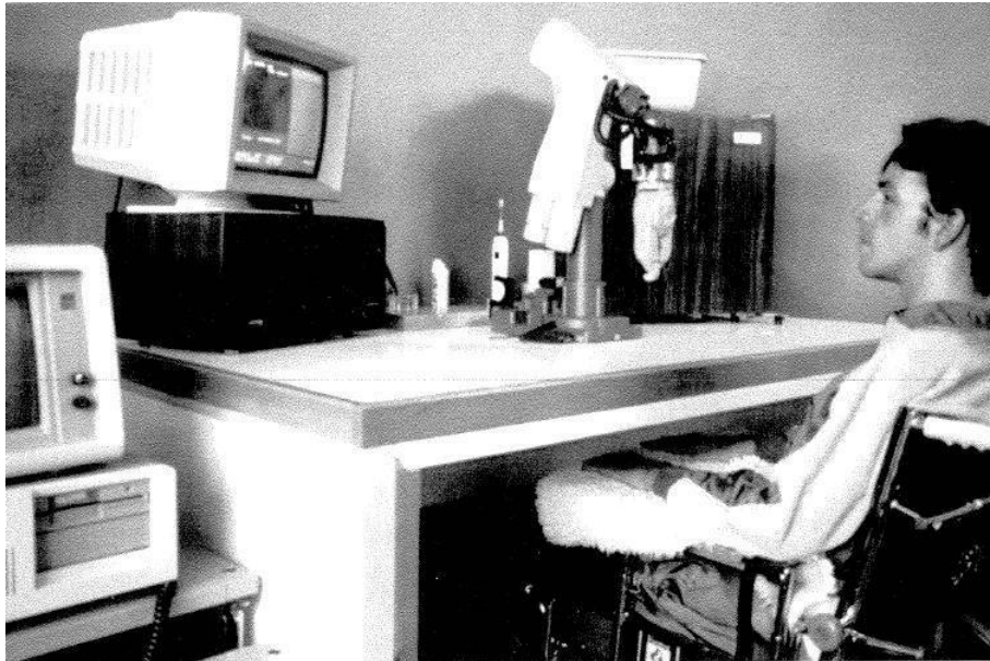
Figure 1.2: The third generation of Desktop Vocational Assistant Robot (DeVAR-III) for helping a patient with disabilities in activities of daily living (ADL). Image courtesy of Hammel et al. [2].
