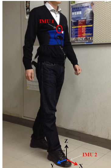
Fig. 2-9: A photo of the testing (IMU 1 is fixed on chest and IMU 2 is fixed on foot).
