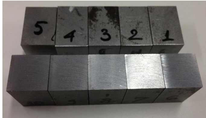
(b) Steel C: 0.45% after preparing surface for machining.
