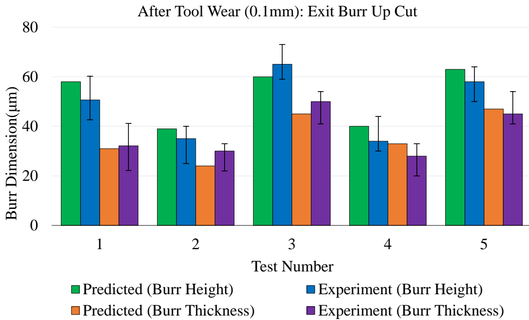
Fig. 5.34 Comparison of exit burrs of steel after tool wear of 0.1 mm.
