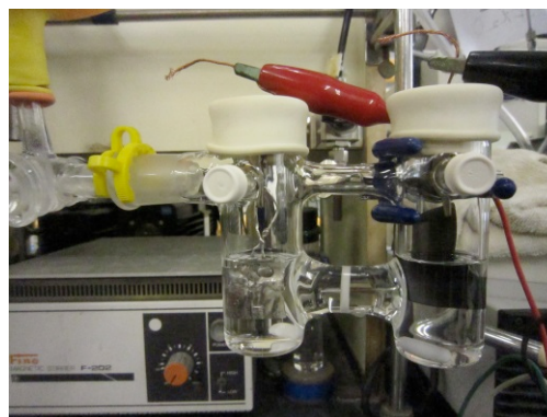
Figure 9. 実験に用いた電解セル (左) Undivided cell、(右) Divided cell
