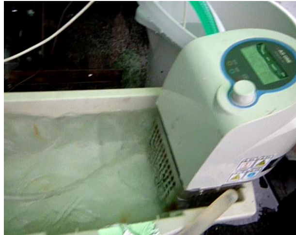
Fig. 20 Hot water tank with electric heater
