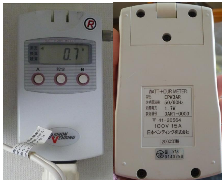
Fig. 33 Watt-hour Meter and its specification
