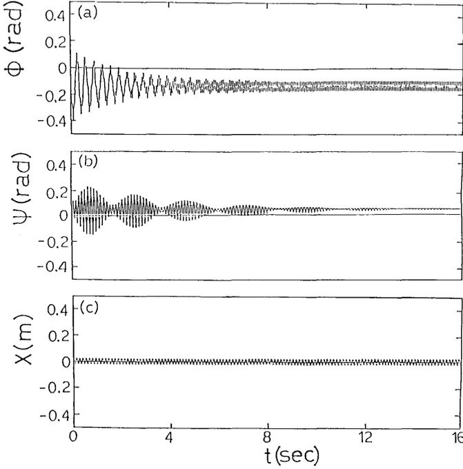
Figure 2. Response of the system for  $X_0=0.023$ [m],  $l=0.076$ [m],  $2\xi_1=1.0$ [1/s],  $2\xi_2=0.5$ [1/s],  $\omega=50$ [rad/s], and  $g=9.8$ [m/s<sup>2</sup>]. (a),  $\phi(t)$ ; (b),  $\psi(t)$ ; (c),  $X(t)$ . Initial conditions:  $\phi(0)=\dot{\phi}(0)=\psi(0)=\dot{\psi}(0)=0$ .
