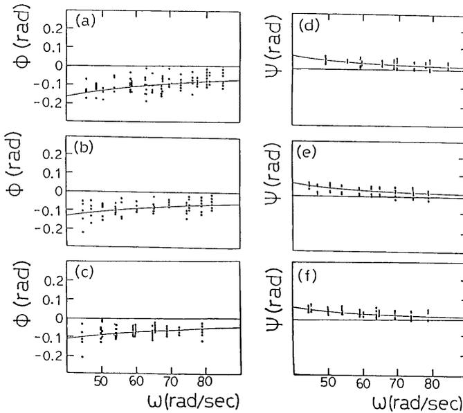
Figure 6.  $\phi$  vs.  $\omega$  and  $\psi$  vs.  $\omega$  in steady state for  $l=0.0760$ [m],  $2\xi_1=1.0$ [1/s],  $g=9.8$ [m/s<sup>2</sup>], and several values of  $X_0$ . (a) and (d)  $X_0=0.0230$ [m]; (b) and (e)  $X_0=0.0290$ [m]; (c) and (f)  $X_0=0.0350$ [m].  $\circ$ , Experimental; —, theoretical.
