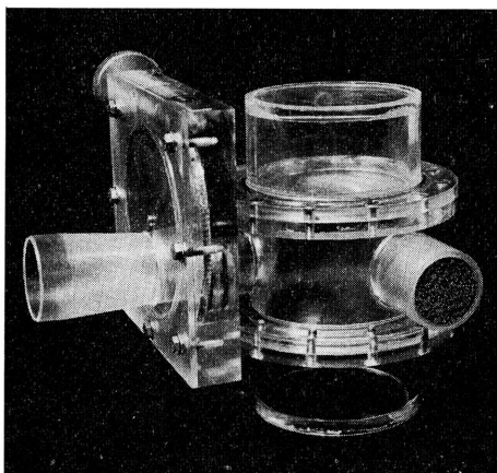
Fig. 6. Integrated assembly of the elements Z_2 , Z_8 and Z_4 with the adjusting mechanism of resistance R_4 .
