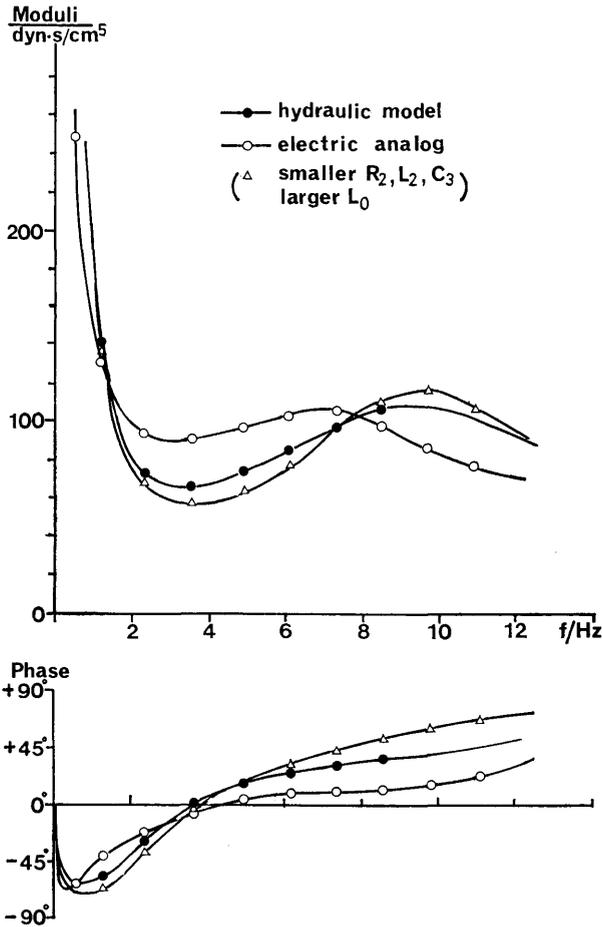
Fig. 12. Effect of different  $L_0, R_2, L_2$  and  $C_3$  on the input impedance for systemic circulation, estimated by electric analog model ( $\Delta$ ). Black dots represent the measured input impedance of hydraulic model, and the original theoretical values are described by circles (See in text).
