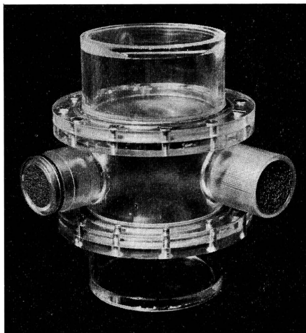
Fig. 2. Integrated design of the elements Z_2 , Z_3 and Z_4 for the systemic circulation
