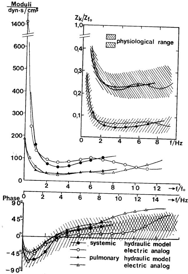
Fig. 10. Input impedance spectra and phase characteristics of the hydraulic and electrical analog model compared with physiological data.
