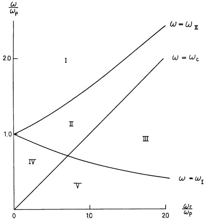
**Fig. 1.** Regions of propagation of the electromagnetic wave. The frequencies  $\omega_I$  and  $\omega_{II}$  are the cut off frequencies for left-handed and right-handed circularly polarized wave,  $\omega_c$  is the electron cyclotron frequency. The right-handed wave can propagate in III, V and I; and the left-handed wave in I, II and III.
