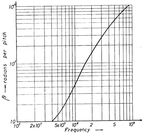
Fig. 3. Frequency characteristics of the Phase Constant  $\beta$ .
