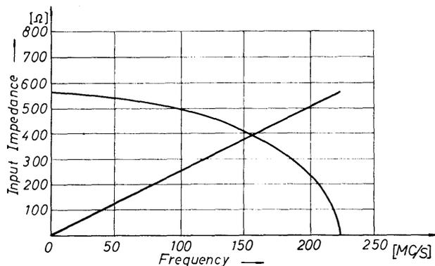
Fig. 8. Frequency characteristics of the input impedance.
