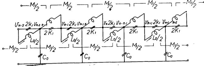
Fig. 5. Equivalent Circuits of the Helix.
