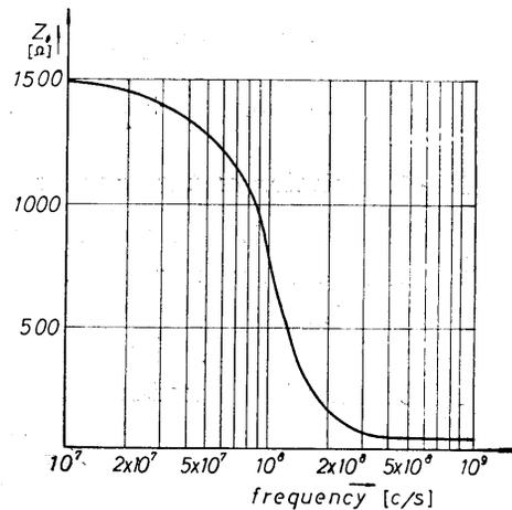
Fig. 4. Frequency characteristics of the characteristic impedance properties.
