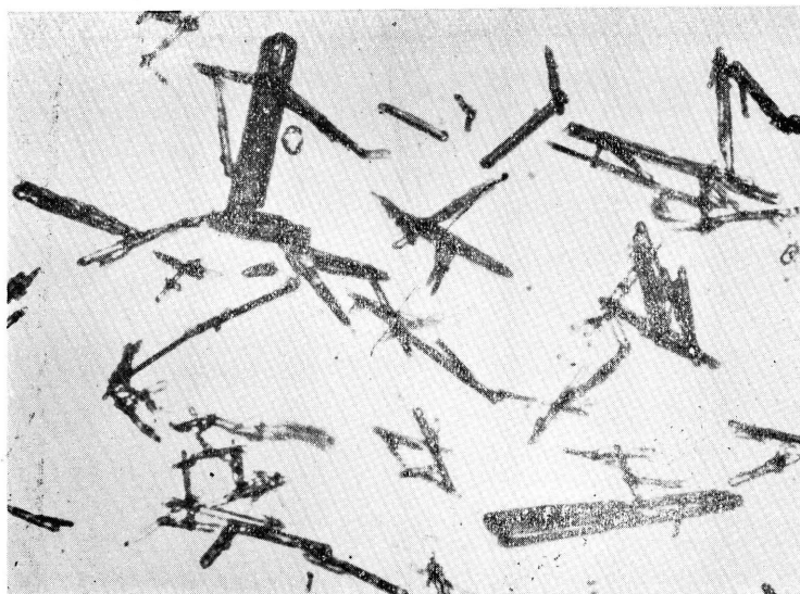
Fig. 1a. Microphotograph of the magnesium carbonate prepared at 50°C. ( \times 200 ).
